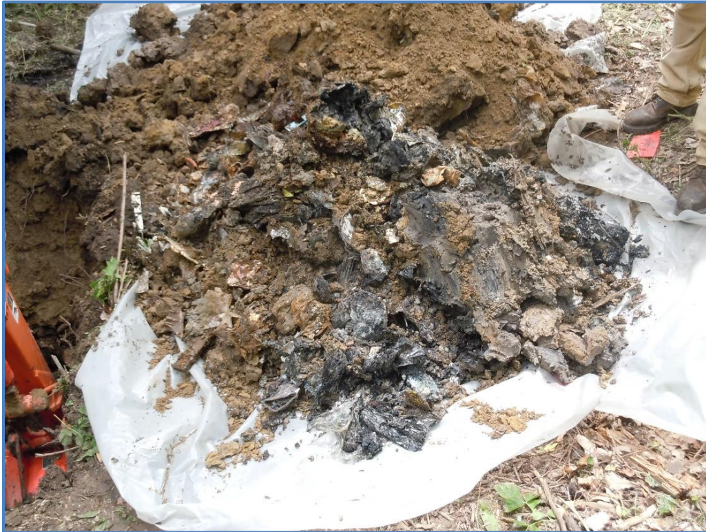
Figure I-11. Photo showing landfill waste from a test pit completed on the main Niagara Sanitation landfill property. Photo taken by Steven Moeller on June 7, 2021.
