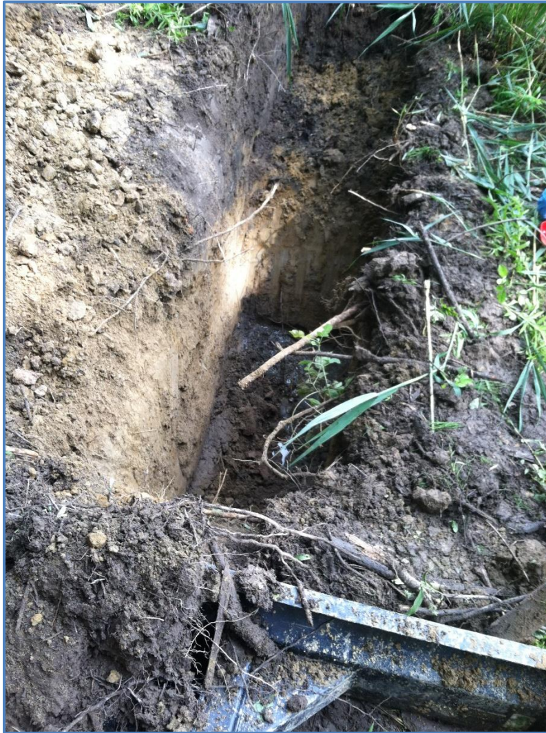
Figure I-19. Photo showing the upper sand (yellow-brown) and underlying silty clay (brown) deposits in test pit TP-10 completed along the southern boundary of the Niagara Sanitation landfill. Photo taken by Glenn M. May on July 20, 2017.
