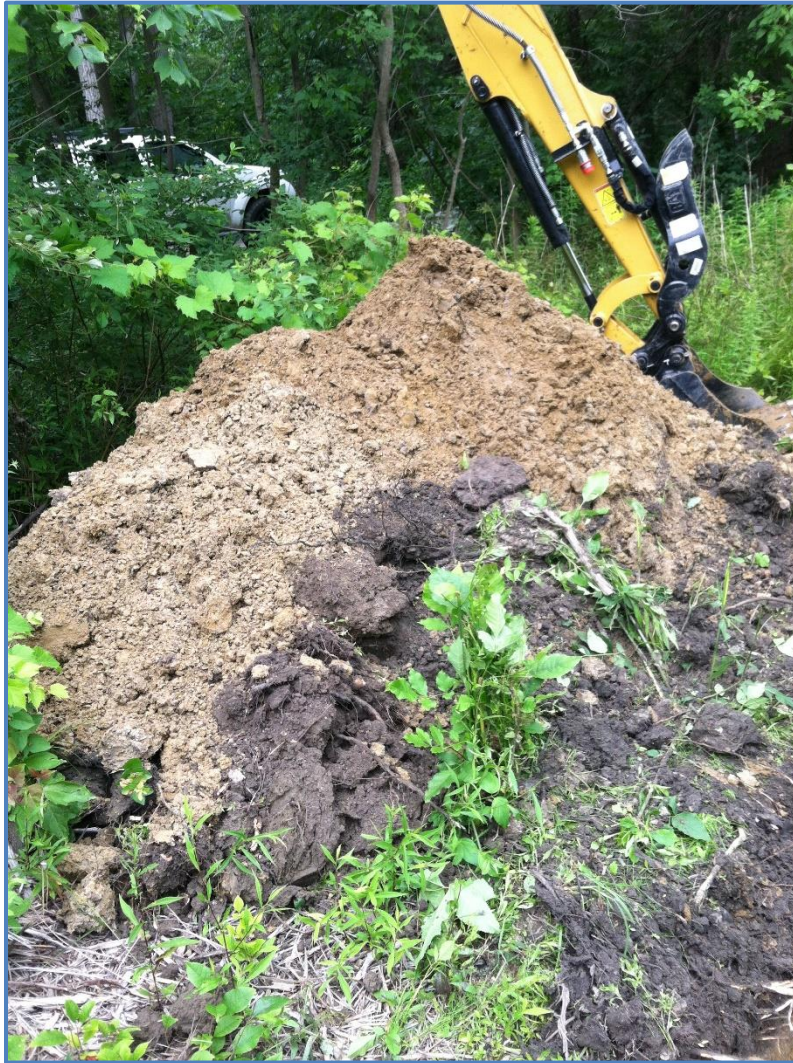
Figure I-16. Photo showing the upper sand deposit (yellow-brown) that was excavated from test pit TP-5. Photo taken by Glenn M. May on July 19, 2017.
