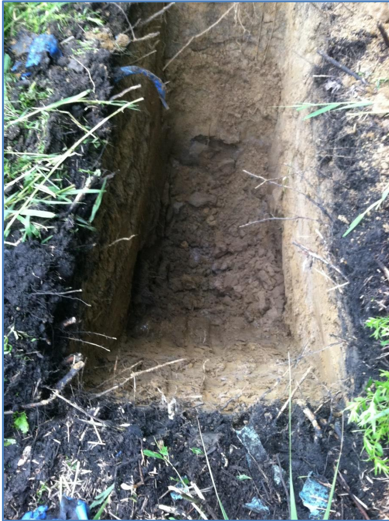
Figure I-17. Photo showing the upper sand (yellow-brown) and underlying silty clay (brown) deposits in test pit TP-9 completed along the southern boundary of the Niagara Sanitation landfill. Photo taken by Glenn M. May on July 20, 2017.
