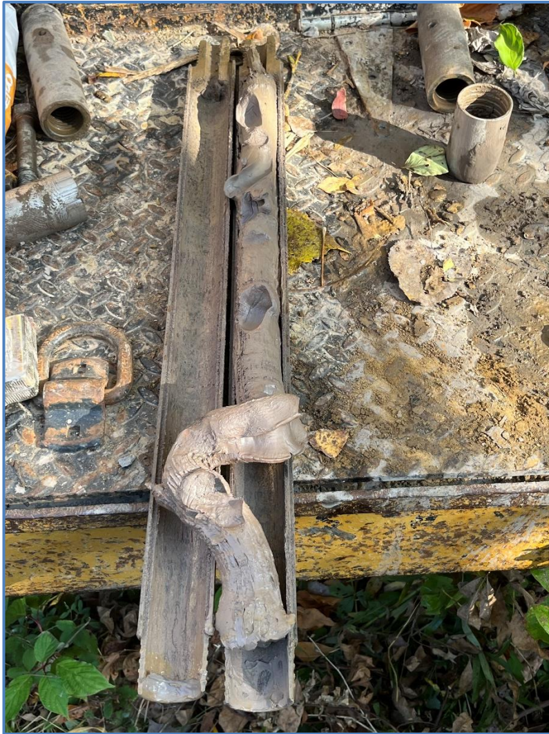
Figure I-24. Photo showing the silty clay deposit from 14' to 16' depth in a split-spoon sample collected from soil boring LPZ-18S. Photo taken by Steven Moeller on October 4, 2023.
