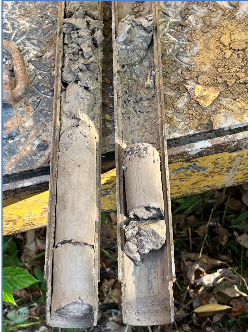
Figure I-23. Photo showing the silty clay deposit from 4' to 6' depth in a split-spoon sample collected from soil boring LPZ-18S. Photo taken by Steven Moeller on October 4, 2023.
