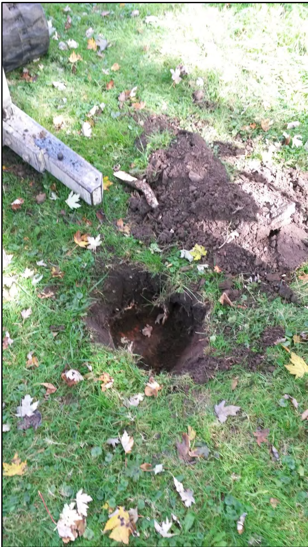
Photo 5: picture of hand dug hole surrounding B-6. Reddish-orange material in hole is the top of the discovered UST.
