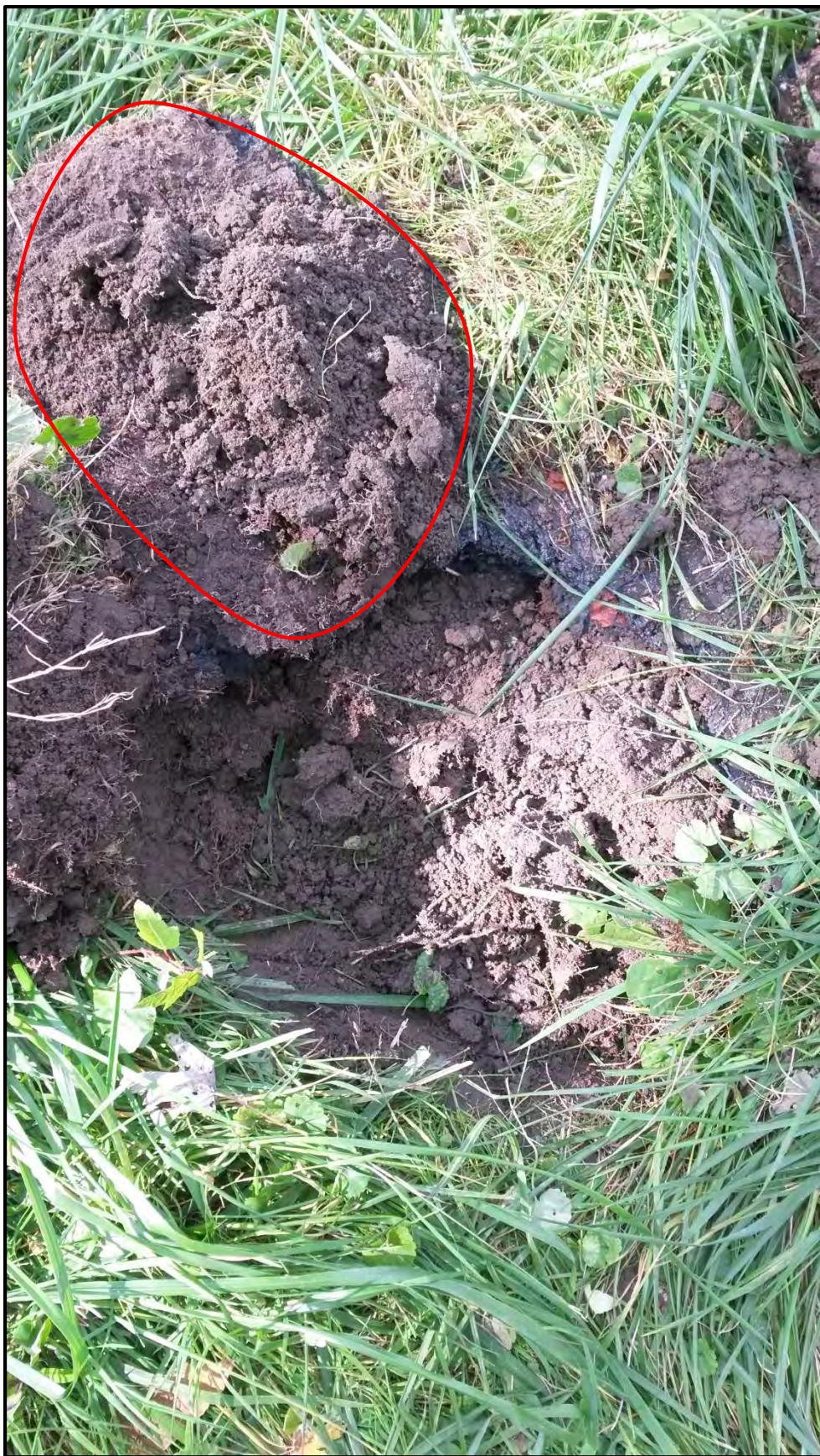
Photo 7: picture of hand dug hole surrounding the tar seep. Note that soil/root layer immediately below the seep does not appear impacted by tar (outlined in red).
