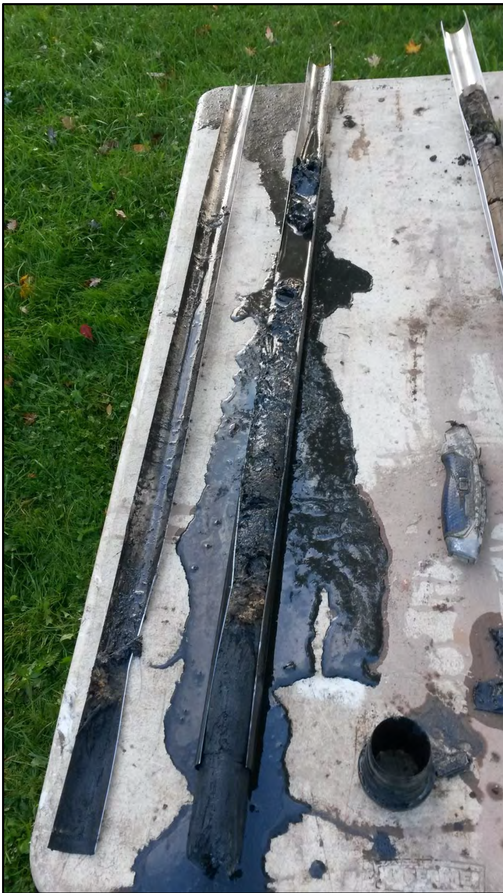
Photo 3: picture of B-2 from 4'–8' core. Note high moisture content and black material throughout. Very strong sewage smell. Refuse debris evident in the middle portion of the core.
