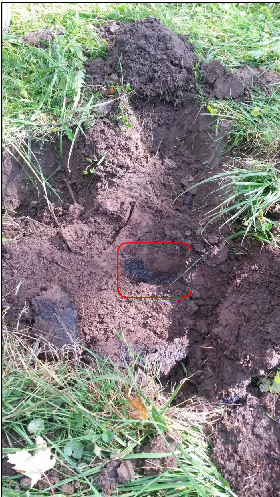
Photo 9: picture of hand dug hole surrounding the tar seep, below surface soil. Note the 'vein' of tar that appears to be the migration pathway to the surface (outlined in red).
