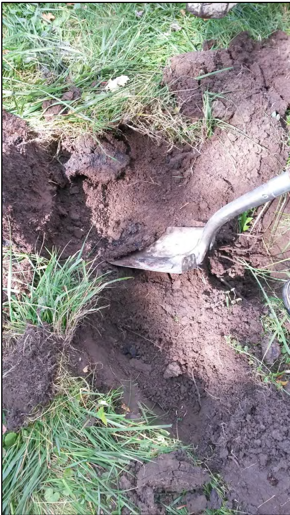
Photo 8: picture of hand dug hole surrounding the tar seep, below surface soil. Note that tar impacts are not widespread.
