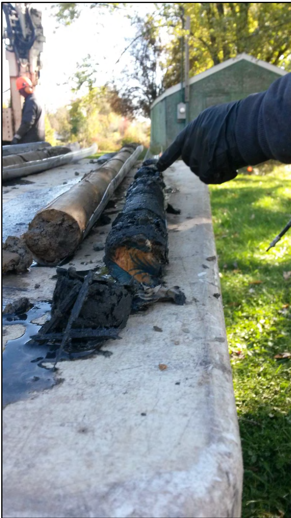
Photo 4: picture of B-4 from 4'–8' core. Note woody debris mixed with refuse material. Apparent wall paper in the end of the core. Very strong sewage smell. Black discoloration throughout.
