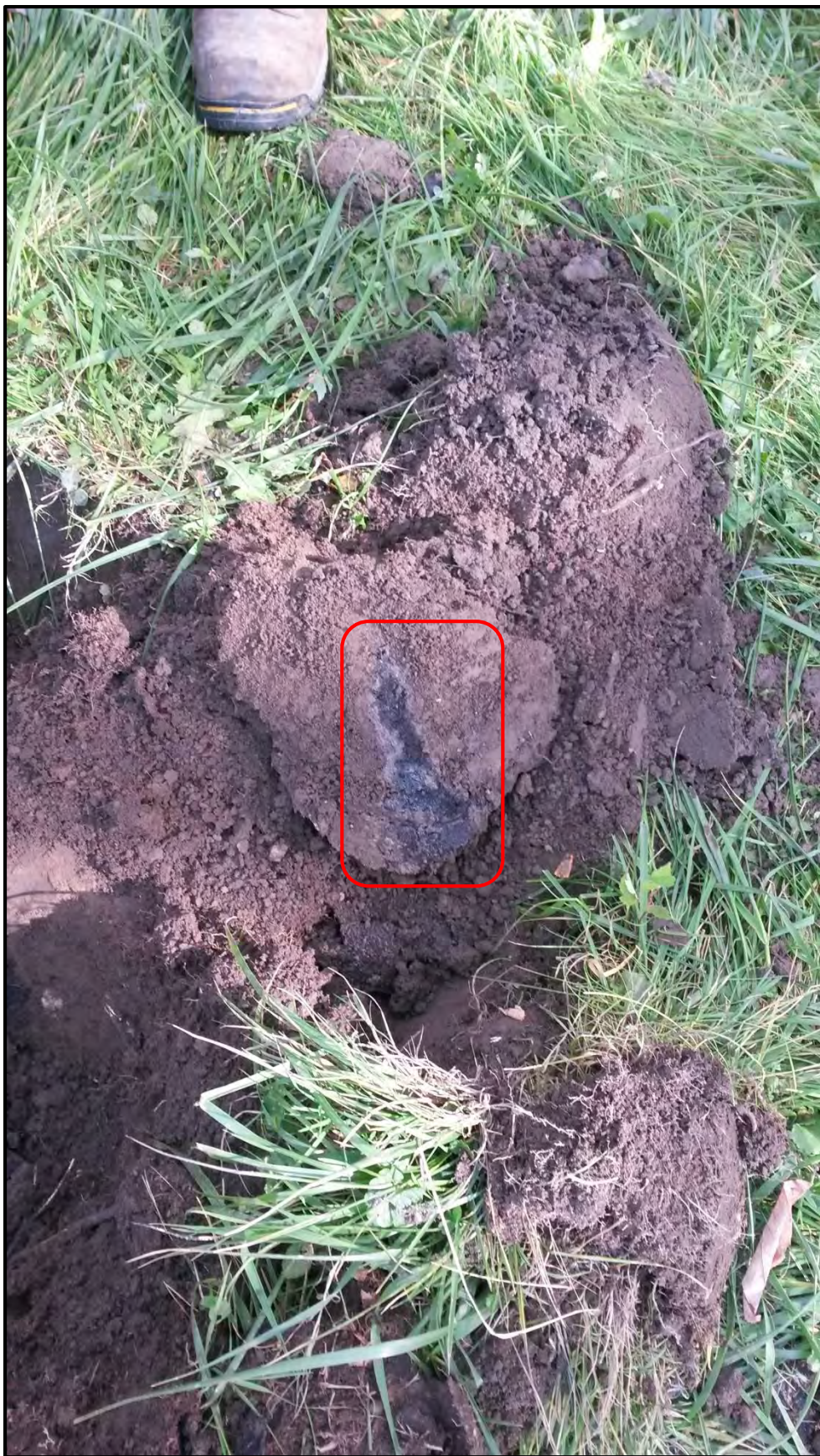
Photo 10: picture of a horizontal shovel recovery from under the tar seep. Note the 'vein' of tar that appears to be the migration pathway to the surface (outlined in red).
