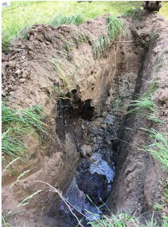
Photo 1 - Test Pit 1, note vein with potential tar.
