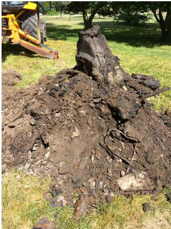
Photo 4 - Test Pit 2 waste stockpile.
