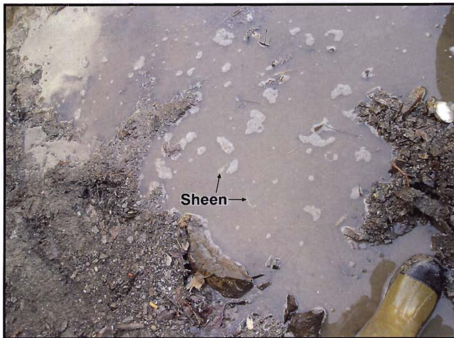
Photograph 5: Sheen observed when sediments agitated in the vicinity of TS-10.
