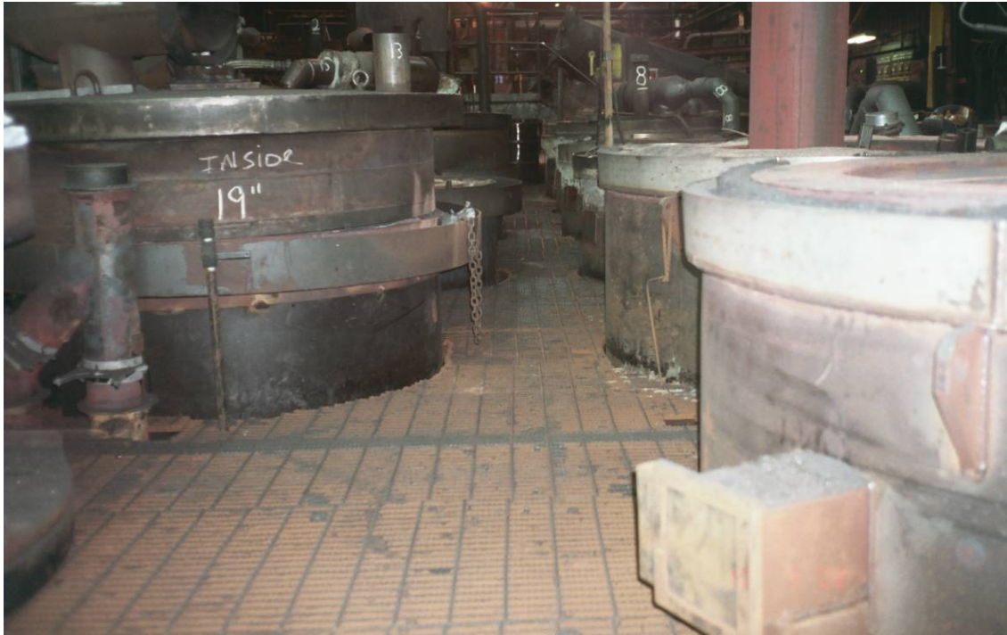
Photograph 3: Vault 1 (bake pit). The grated floor covers the vault. The large cylinders are furnaces that stand vertically in the vault.
