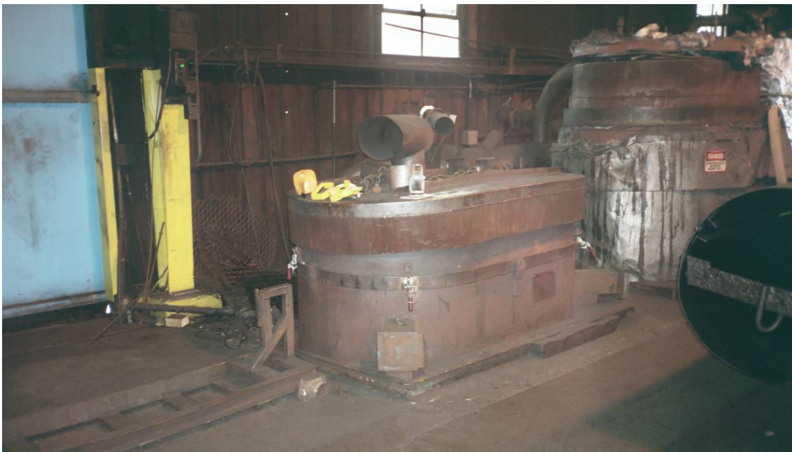
Photograph 4: Vault 2 (preheater vault). The preheater fills most of the vault volume. The steel rim of the vault is visible adjacent to the floor.
