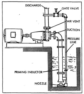
FIGURE 34. PRIMING BY INDUCTOR
