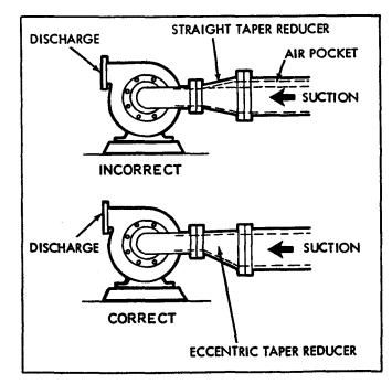
FIGURE 23. AIR POCKETS IN REDUCER
