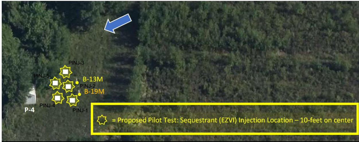
FIGURE 3: GENERAL INJECTION IMPLEMENTATION – INJECTION LOCATIONS P-4
