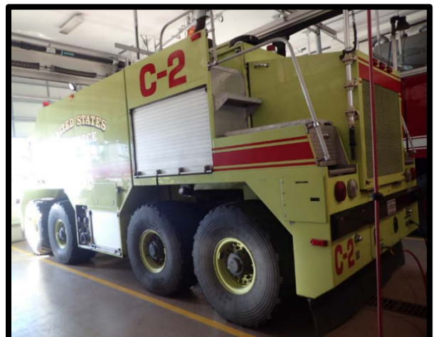
Photo 6 Crash 2 (left side), Model P-23, 300-gallon AFFF tank.
