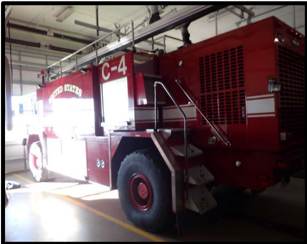
Photo 3 Model P-23, 300-gallon AFFF tank.
