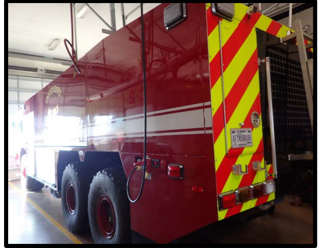
Photo 8 VLP Model, 400-gallon AFFF tank.
