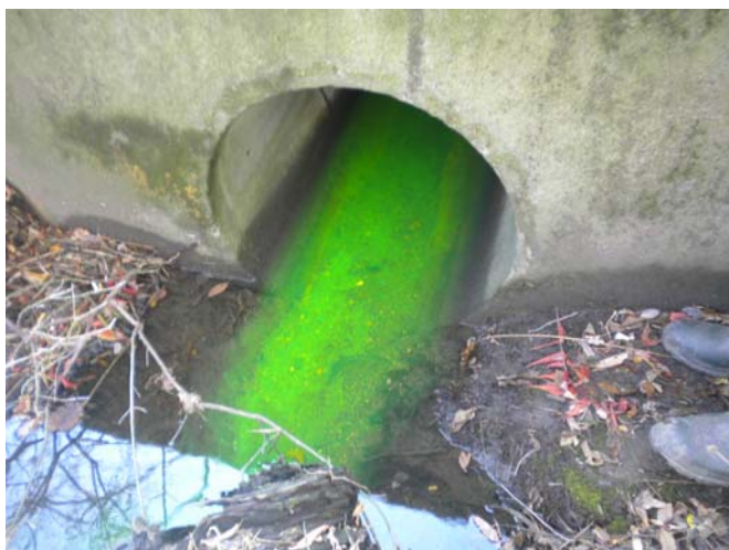
Dye testing from bulkhead outfall
