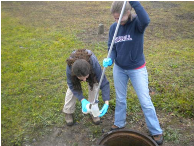
Manhole water sampling with dipper
