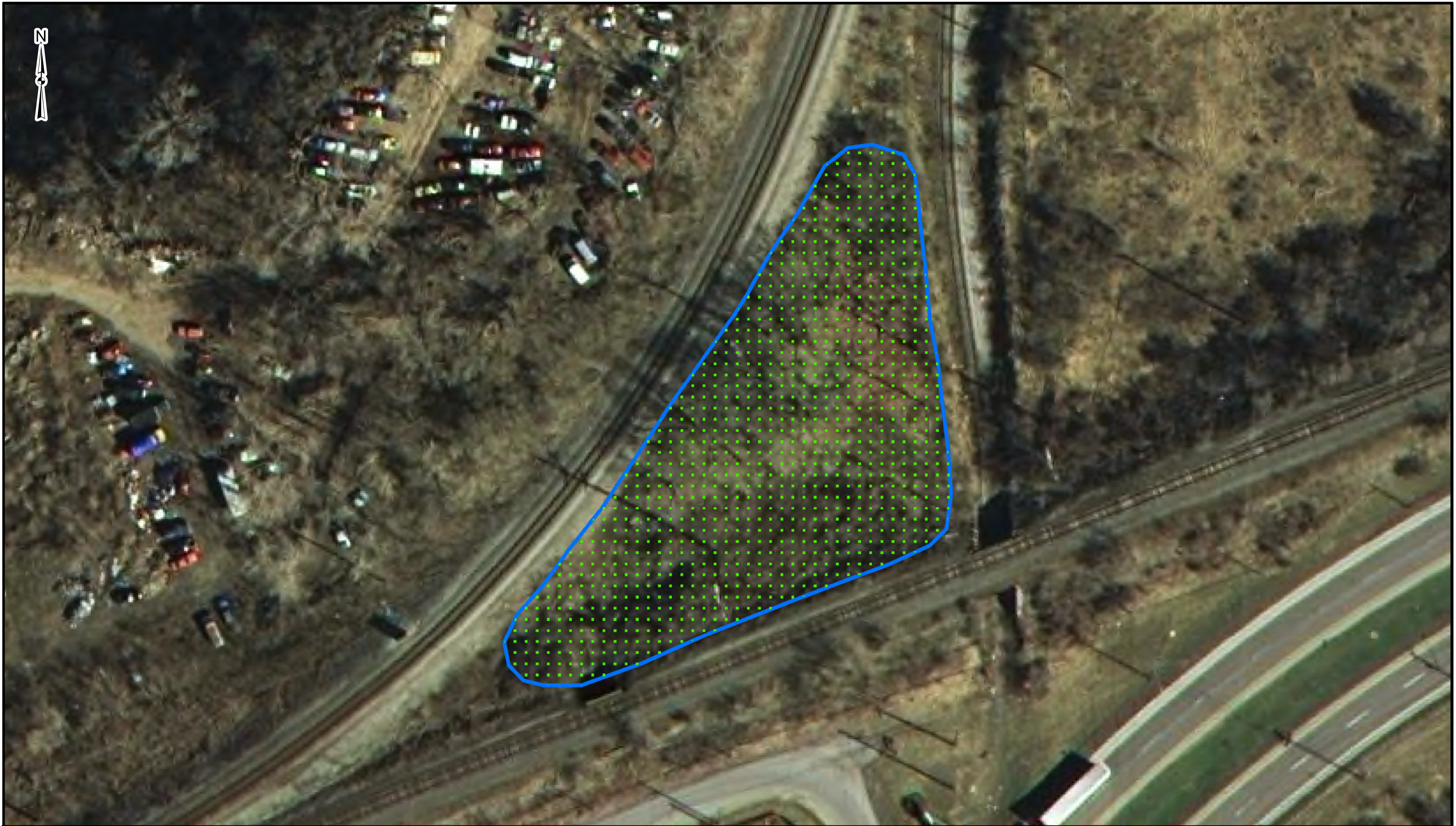
FIGURE 6-3 OU3 Alternative 3: Landfill Capping
