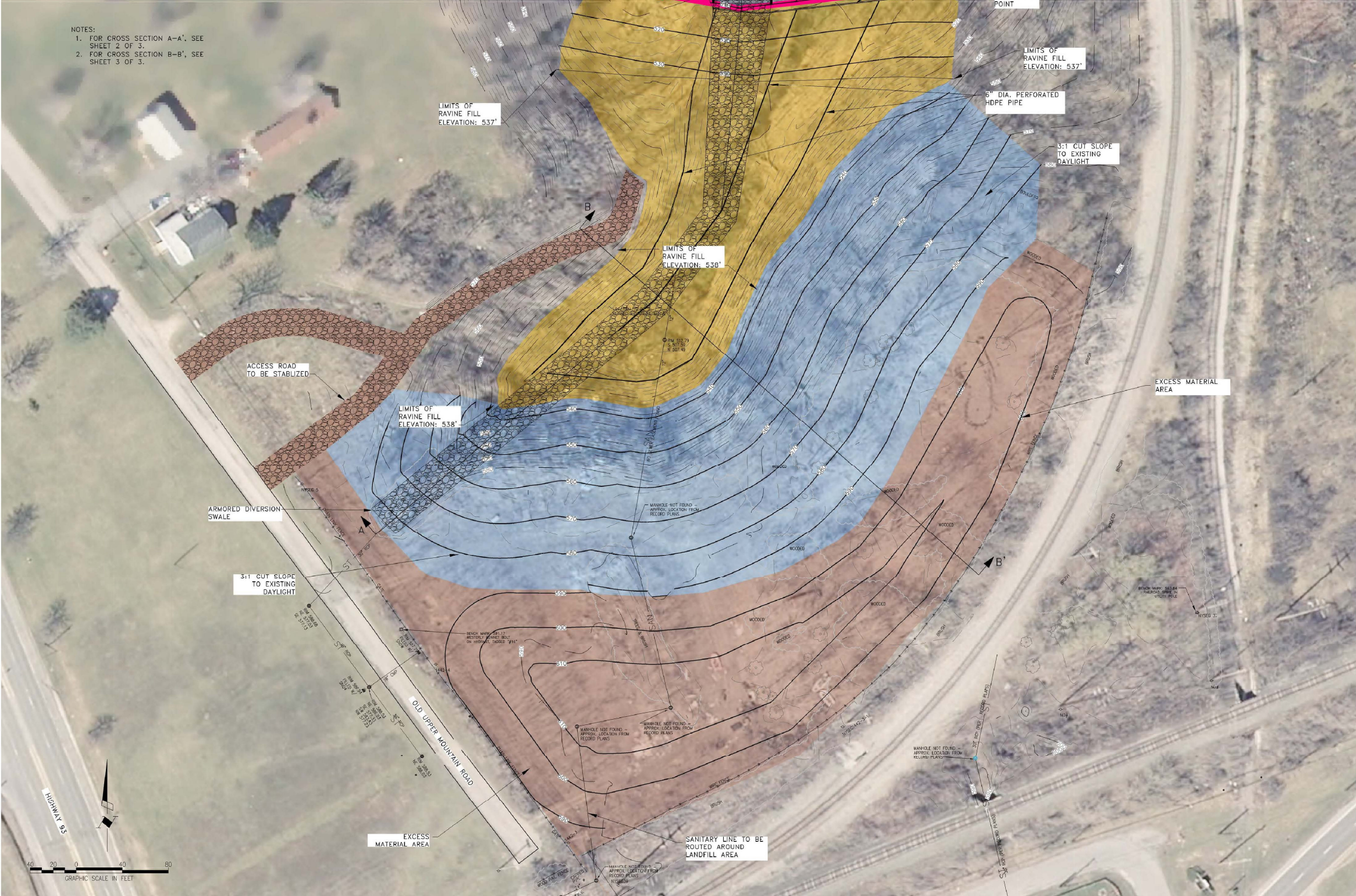
FIGURE 6-4 OU 1 Alternative 5 and 6: Landfill Capping- Extended Landfill Footprint
