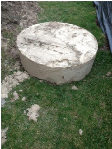
4/16/2013: Concrete core from Outfall D002 Headwall
