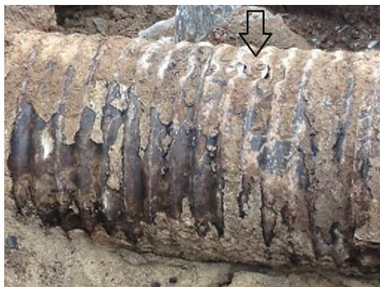
7/1/2013: Hole observed on top of GMCH sanitary sewer line
