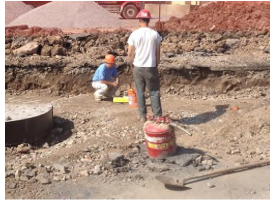
5/22/2013: Density testing by SJB on backfill in vicinity of MH-7 looking south
