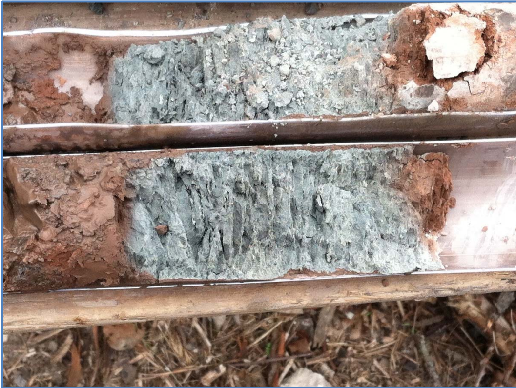
Figure G-8. Photo showing lime waste in a soil boring completed at the Site. Photo taken by Glenn May on July 10, 2013.
