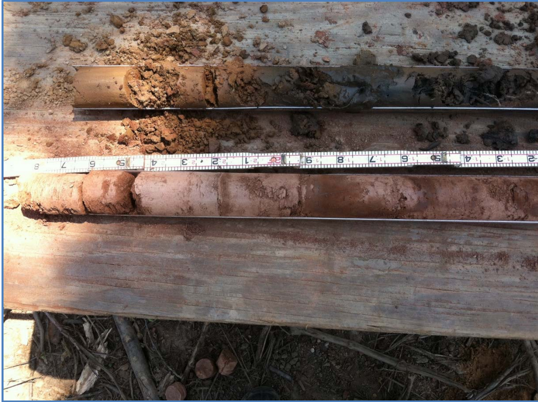
Figure G-10. Photo showing native silty clay in a soil boring completed at the Site. Photo taken by Glenn May on July 16, 2013.
