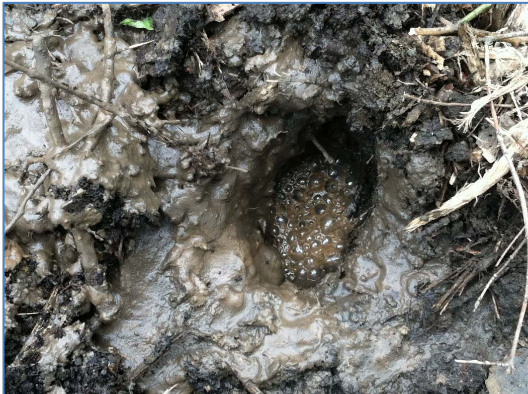
Figure G-13. Photo showing water bubbling in a completed soil boring. This water eventually rose to the surface. Photo taken by Glenn May on July 12, 2013.
