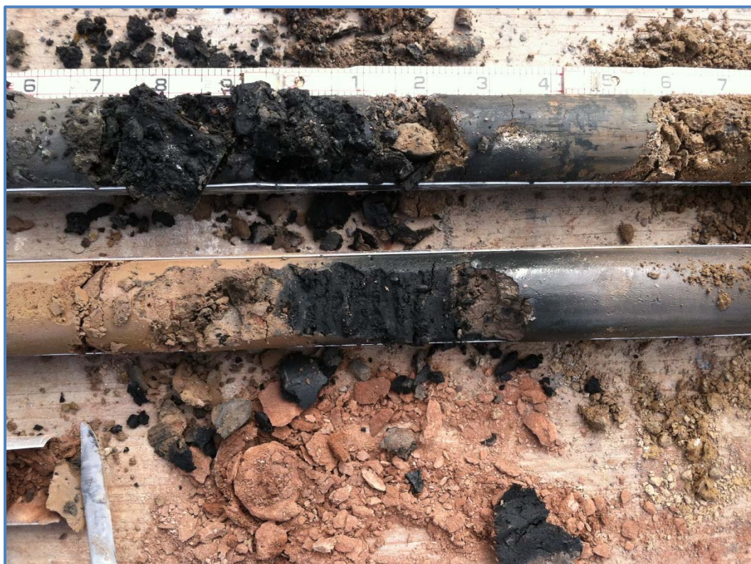
Figure G-9. Photo showing black sludge in a soil boring completed at the Site. Photo taken by Glenn May on August 6, 2013.
