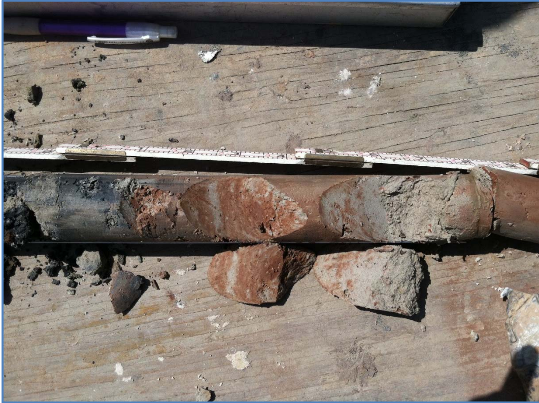
Figure G-12. Photo showing mottling in native silty clay in a soil boring completed at the Site. Photo taken by Glenn May on August 5, 2013.
