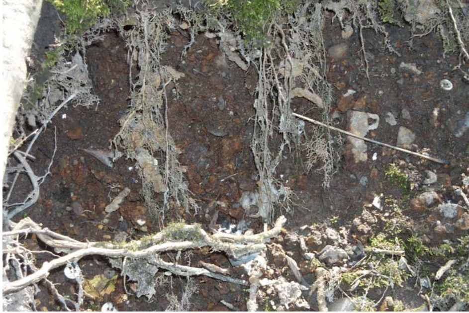
Figure 5-3. Closeup photograph of ash fill in the creek bank along Eighteenmile Creek. Observe the buttons, which are characteristic of the ash fill on the island of the former Flintkote property. Photograph taken by Paul Dicky on April 16, 2002.
