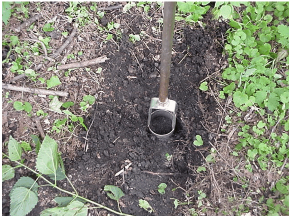
Figure 5-6. Closeup photograph of the slag and cinder fill on the White Transportation property. Photograph taken by Glenn May on September 22, 2005.
