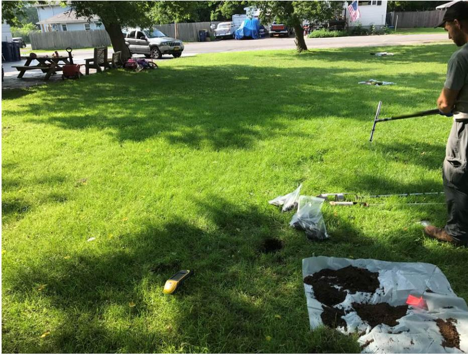
**Photograph 14:** View facing north of a soil boring location at Property P004. RST 3 personnel utilized stainless steel augers to advance soil borings at selected sample locations throughout the nine designated properties.
