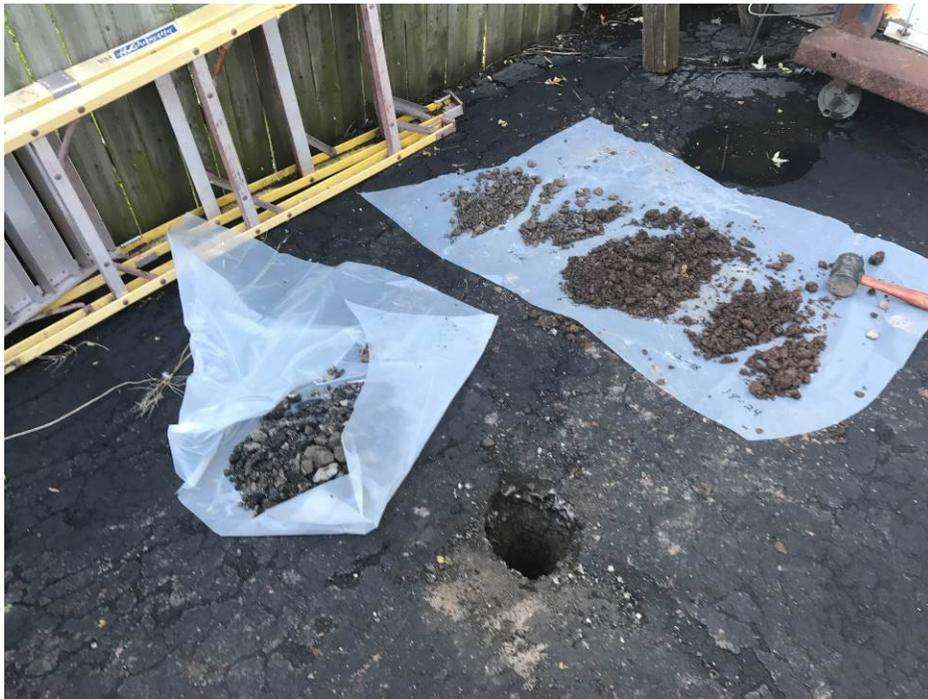
**Photograph 19:** View of the asphalt (left) and soil (right) removed from a boring located on the driveway of Property P023.
