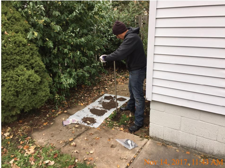
**Photograph 9:** View of RST 3 personnel advancing a boring with a stainless steel auger at Property P034.
