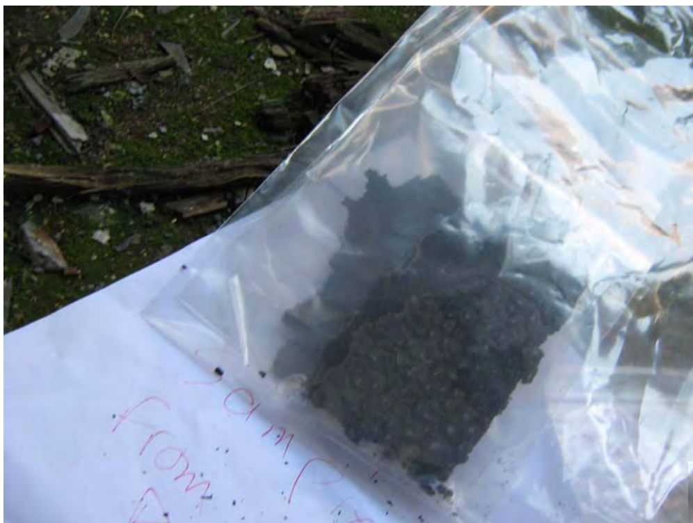
Photograph 6 – Sample PC1-B-AS-05 is roofing material that was submitted for asbestos analysis.
