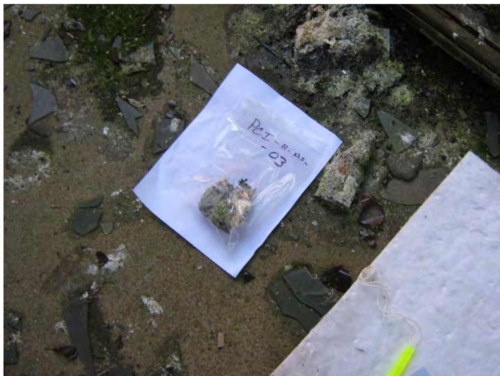
Photograph 4 – Sample PC1-B-AS-03 collected from PACM on the floor and submitted for asbestos analysis.
