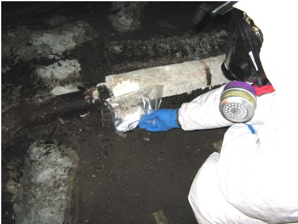
Photograph 8 – Sample No. PC2-BK-AS-01 collected for asbestos analysis.
