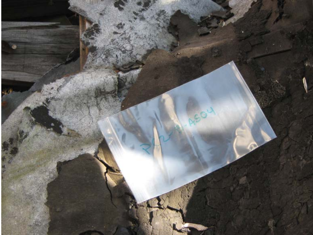
Photograph 15 – Roofing material that had fallen from the roof of the shed. Sample No. PC2-B-AS-04 was collected from here for asbestos analysis.
