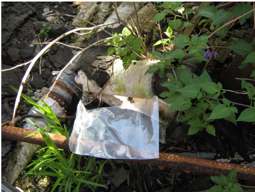
Photograph 14 – Pipe insulation in the area of the shed, northeast of the underground garage. Sample No. PC2-B-AS-03 was collected for asbestos analysis.
