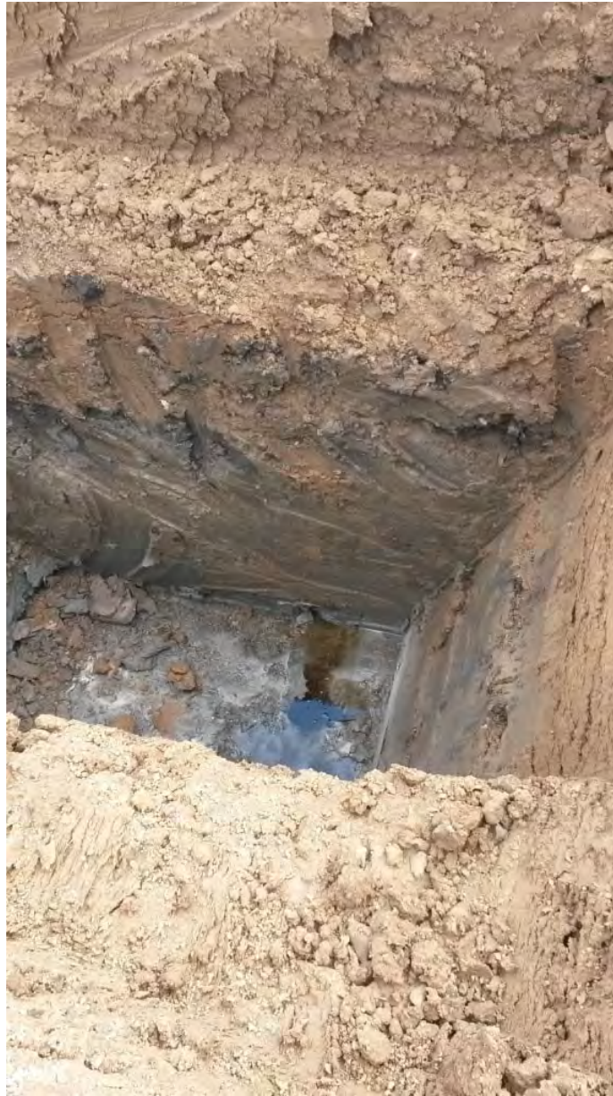
View of test pit LNAPL-20 during advancement on April 24, 2015, showing NAPL impacts.
