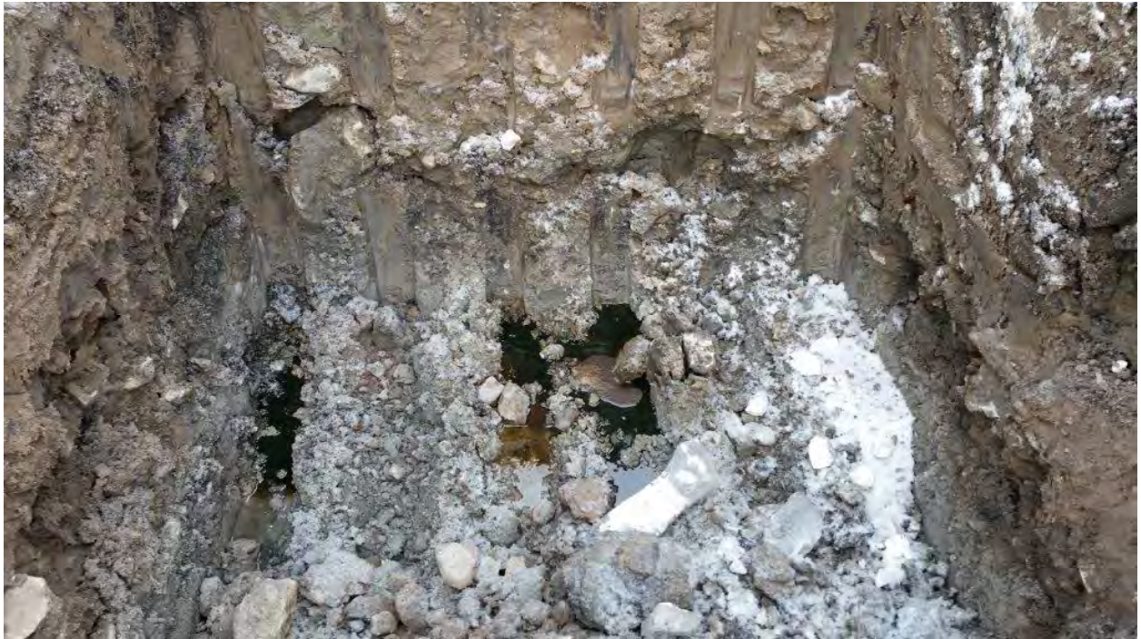
Initial NAPL discovery at test pit LNAPL-1 (T2-E4 location) on February 3, 2015, which was excavated to top of bedrock. (Approximate depth 6 feet below the then current grade). Photo and description provided by AMEC.
