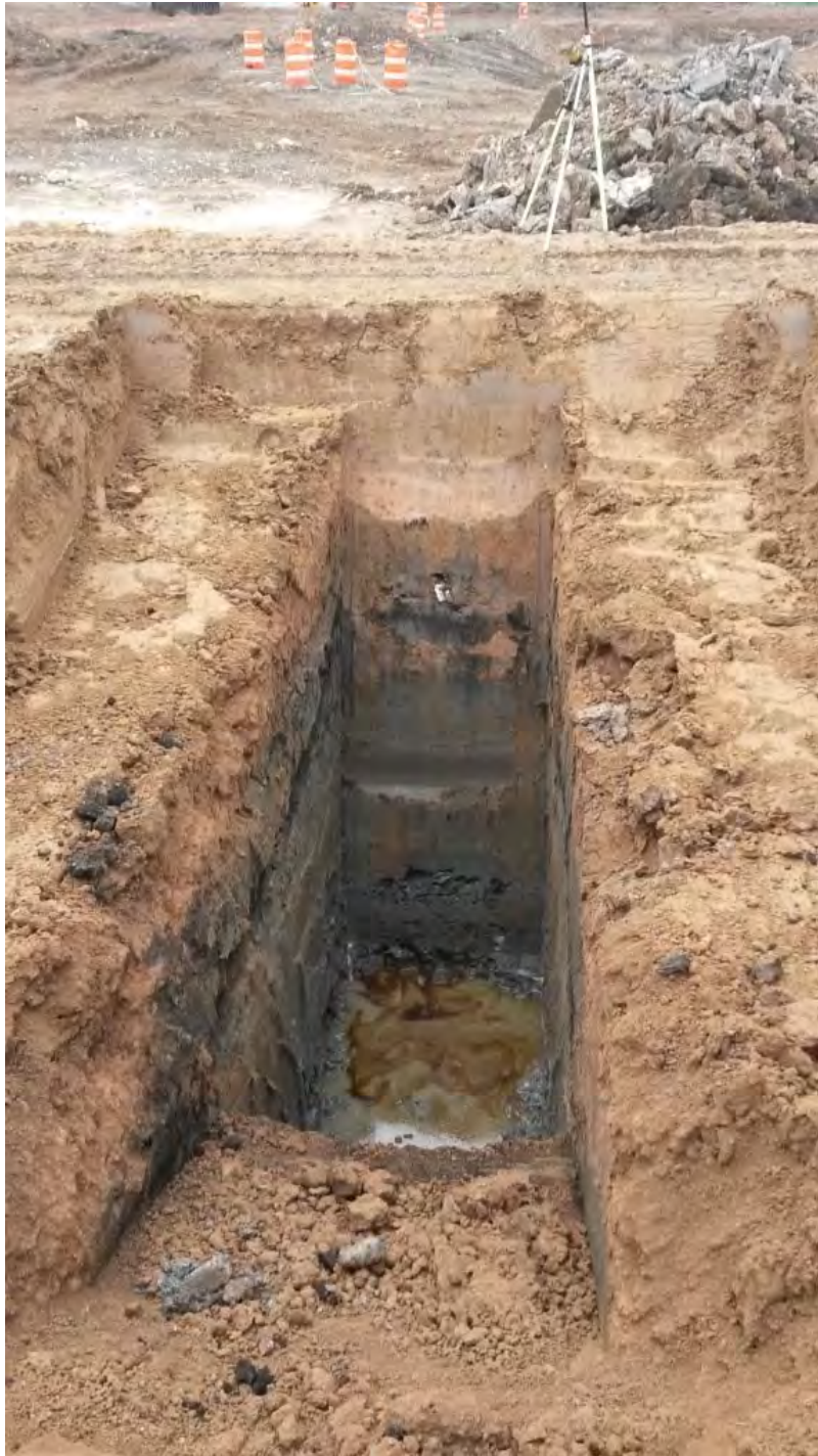
View of test pit LNAPL-24, showing NAPL entering test pit on April 27, 2015.
