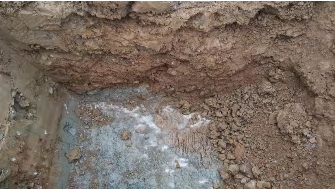
View of test pit LNAPL-15 upon completion on April 23, 2015. No NAPL was observed.
