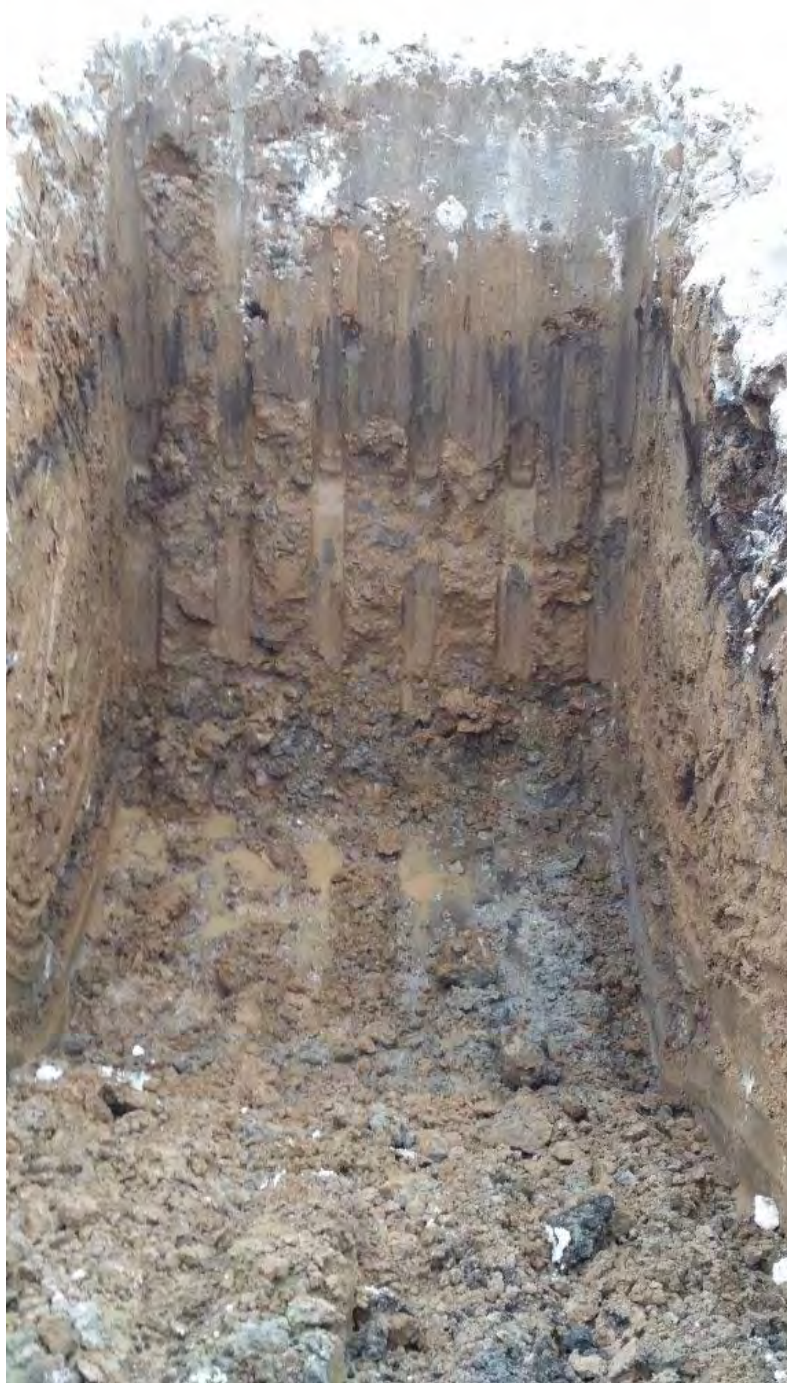
Test pit LNAPL-2 (~25 feet west of LNAPL-1) immediately following excavation on February 10, 2015. Photo and description provided by AMEC.
