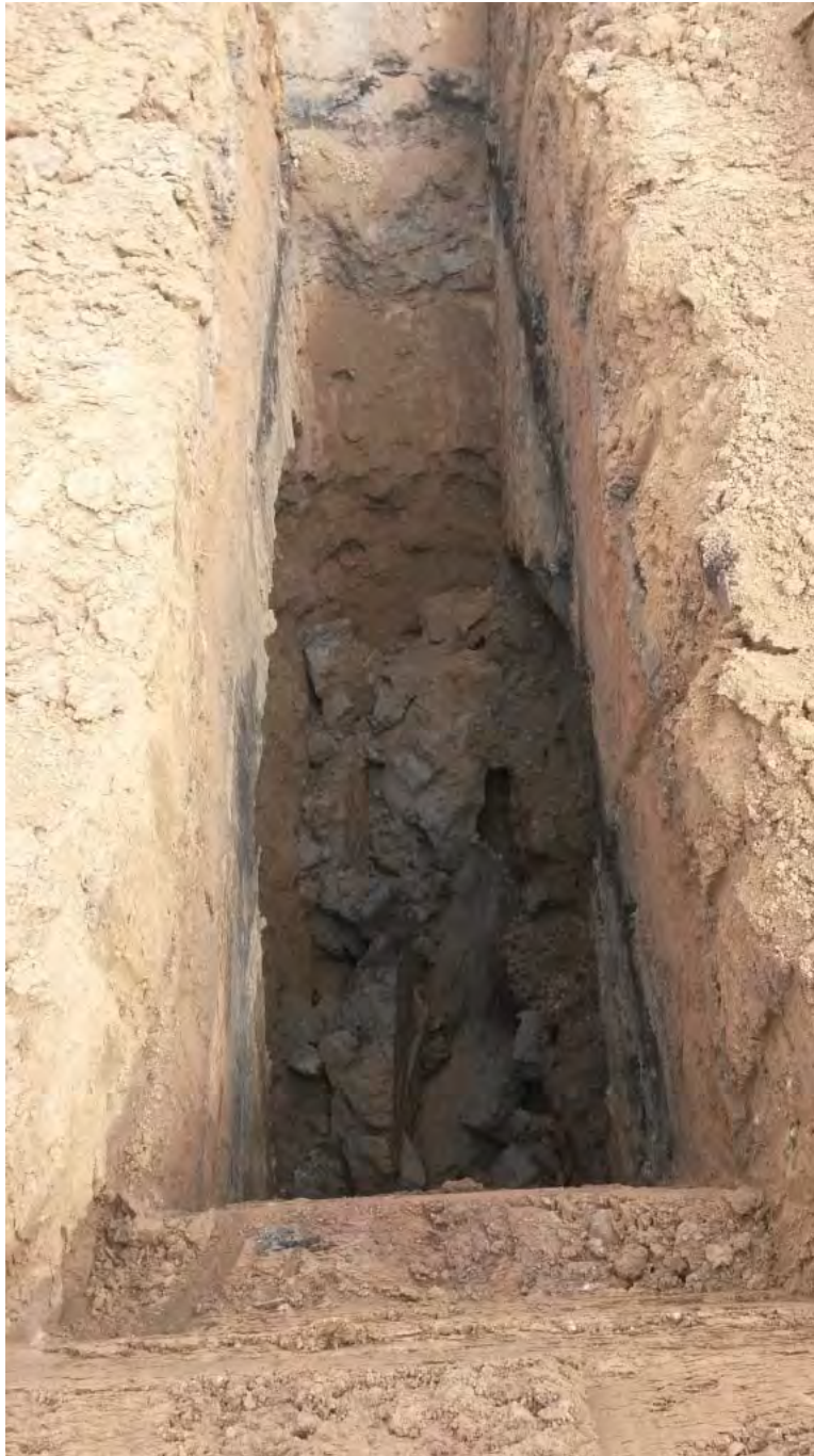
View of test pit LNAPL-23 during advancement on April 27, 2015. The test pit was terminated prior to reaching bedrock due to undermining and caving as shown in this photograph. No NAPL impacts were observed during advancement of the test pit.
