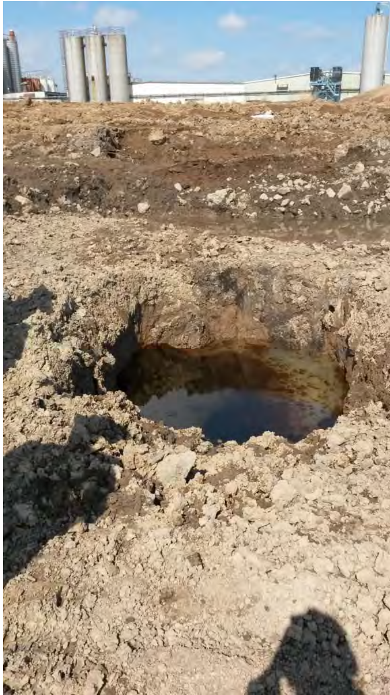
View of test pit LNAPL-2 on March 20, 2015 with NAPL accumulated on surface of water.
