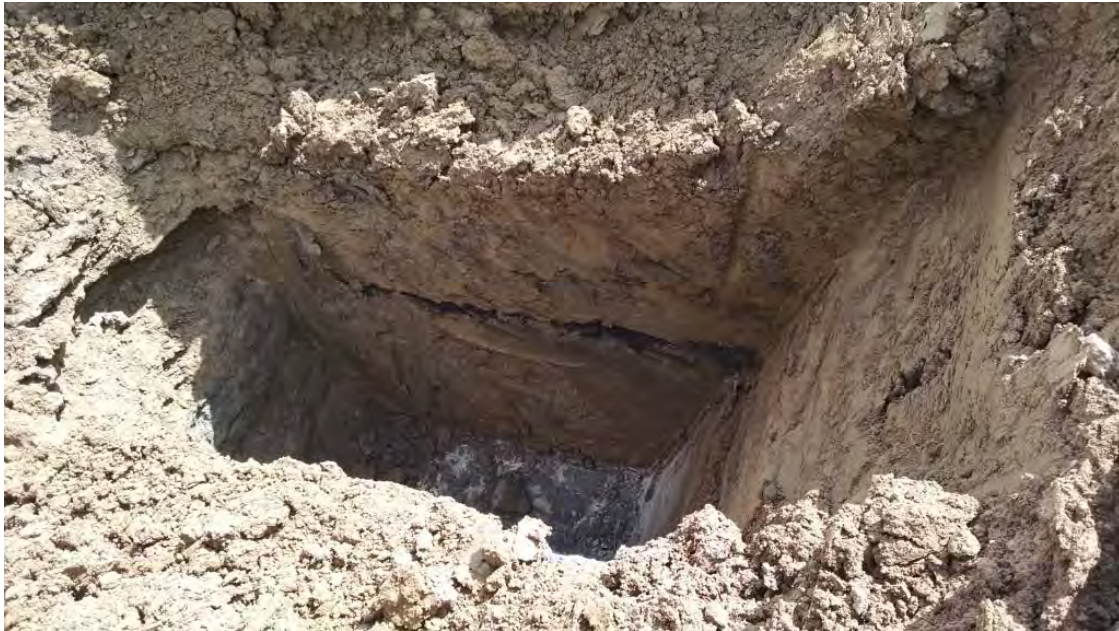
View of test pit LNAPL-11 upon completion on April 23, 2015. No NAPL was observed.
