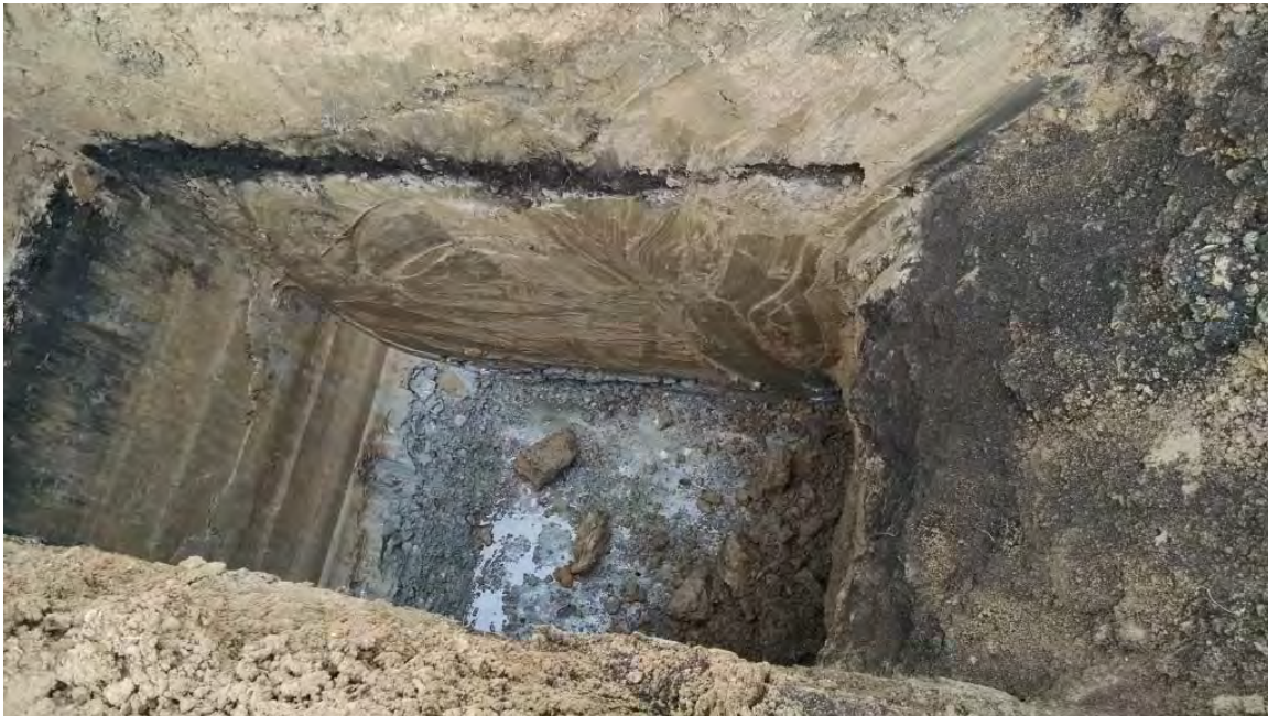
View of test pit LNAPL-12 upon completion on April 23, 2015 showing slight sheen on water at bottom of test pit.
