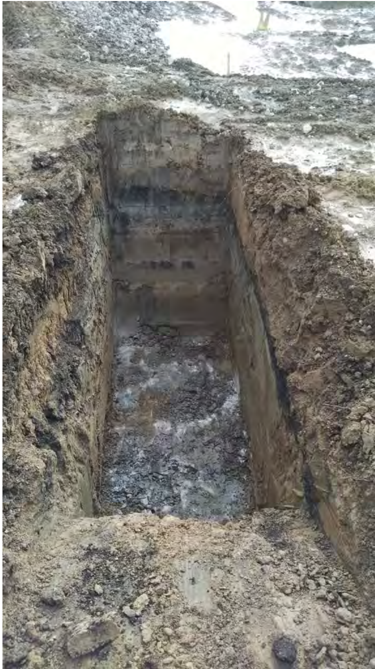
View of test pit LNAPL-10 upon completion on April 23, 2015. No NAPL was observed.
