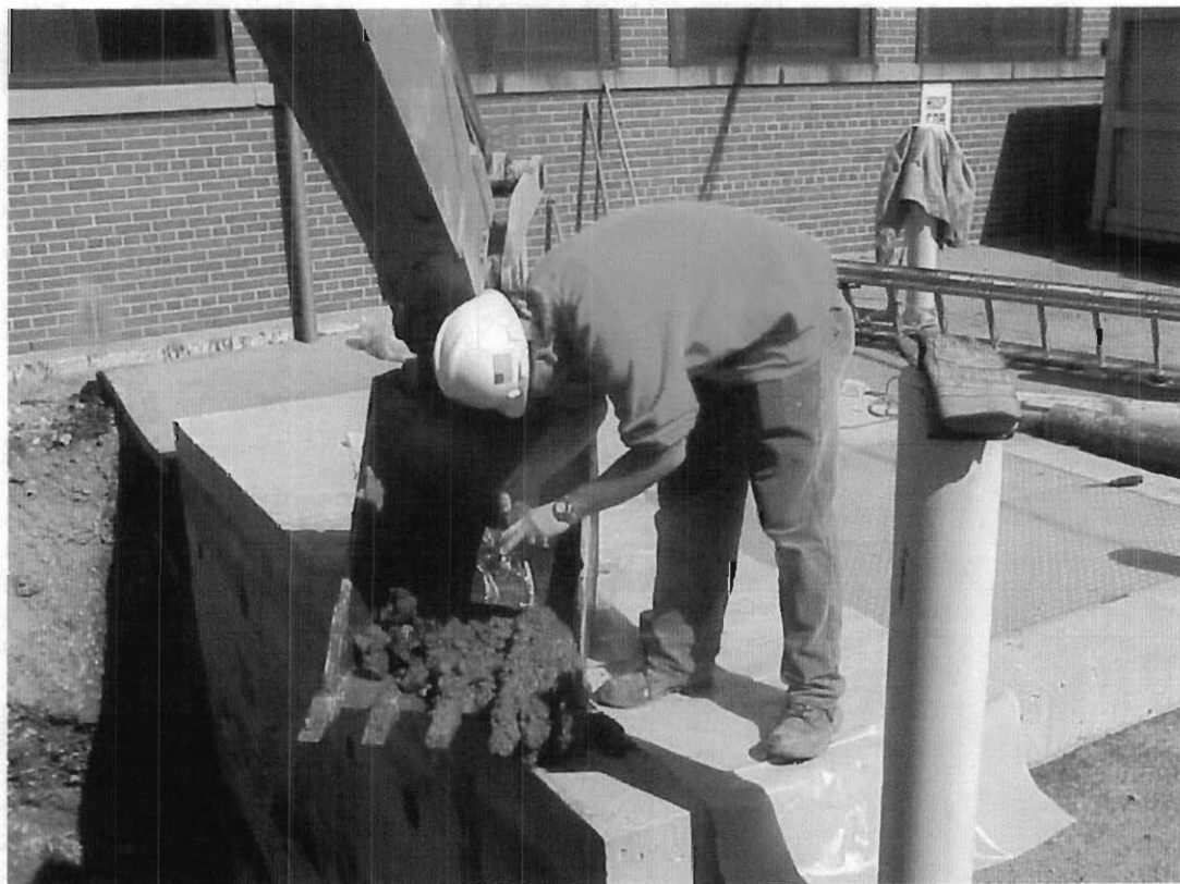
9/22/99 - Collecting soil sample for VOC field screening via headspace analysis with a PID
