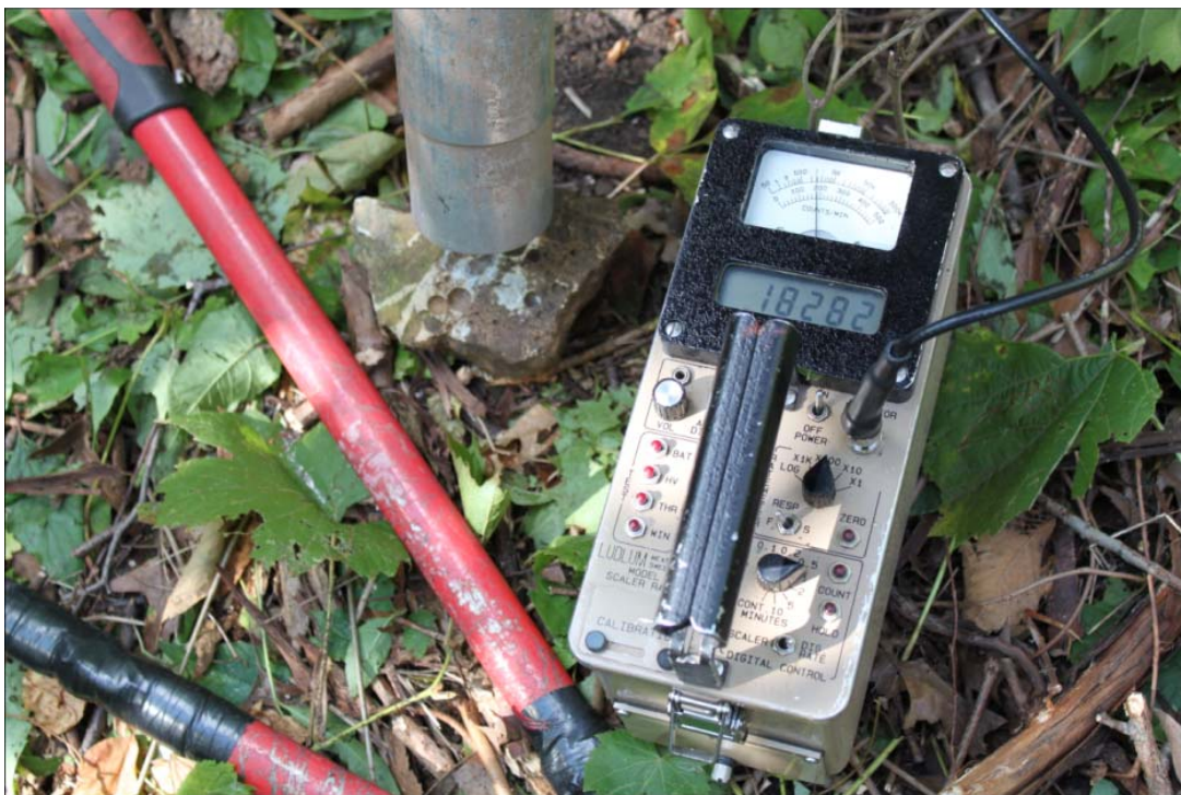
Photo 2 – Rock showing a gamma survey count rate of 18,282 cpm
