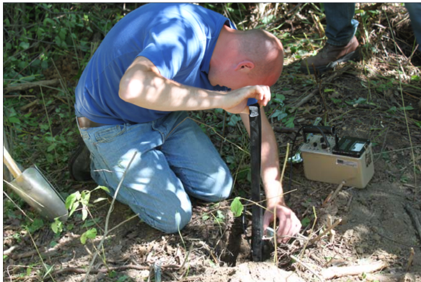
Photo 6 – Lowering Sodium Iodide (NaI) detector into Soil Boring 1 to determine count rates at depth
