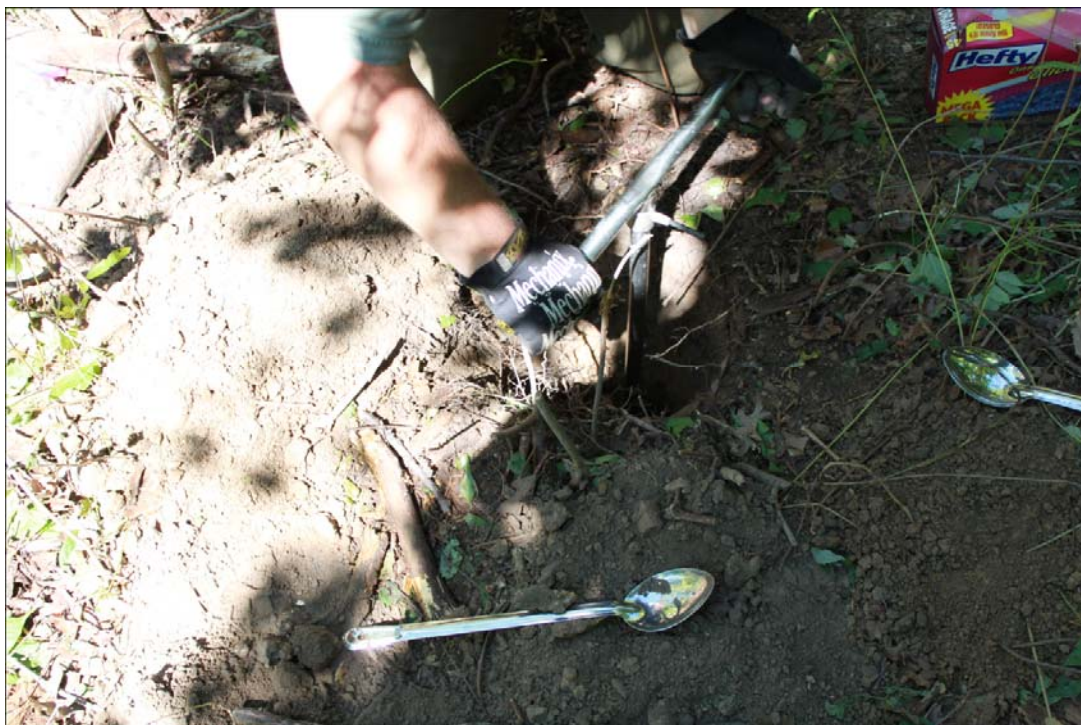
Photo 3 - Advancing hand auger at Soil Boring 1 to a depth of four feet
