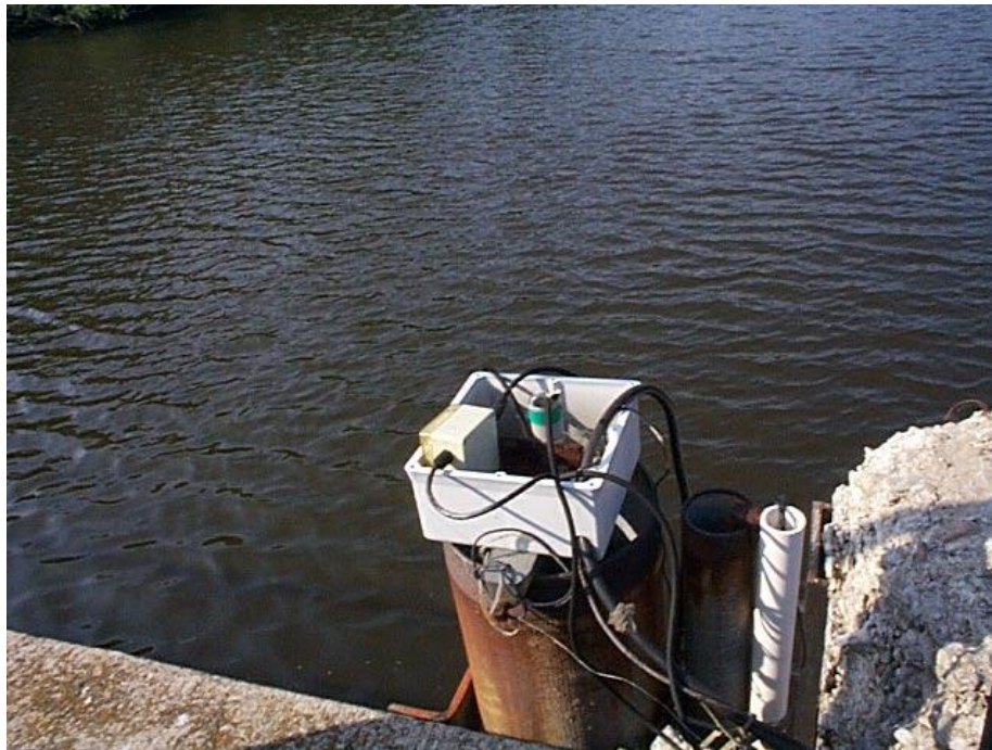
Photo No. 5 - Contents of white box indicate sensing devices on the upstream face of the dam to measure water level.
