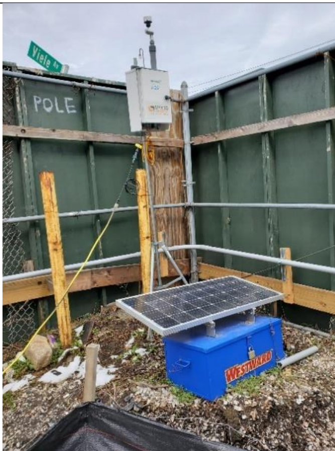
Photo 17 - CAMP probe upwind located northeast of 2.5 acre BUD excavation area
