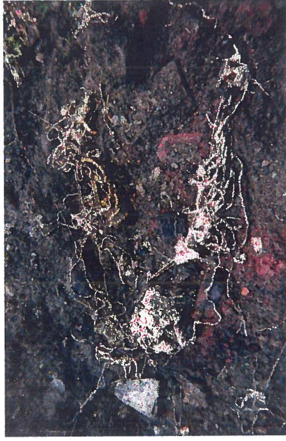
Plastic wire casings in fill materials excavated from test pit TP-10H.
