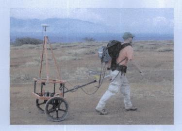
EM-61 being towed along to locate UXOs. Note GPS receiver attached several feet above the top coil. A GPS receiver was not used for this survey.
