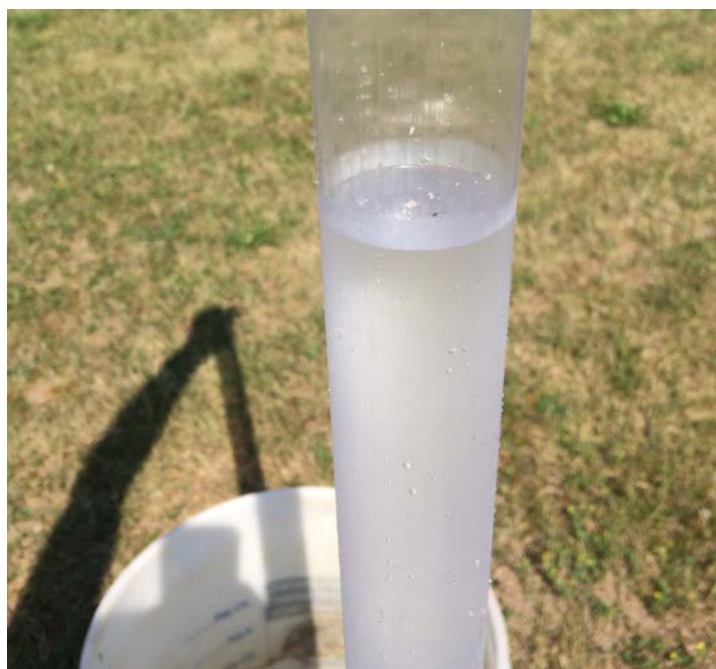
Purge Water from MW-A (no free product observed)
