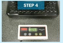
Place KB-1<sup>®</sup> vessel on scale and record the weight
