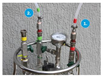
**1. Gas In:** The inert gas tubing remains in the pressurization port (**RED**) for the duration of the injection.
