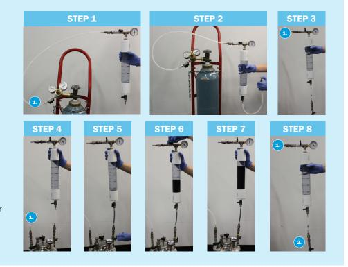
**Step 1:** Cut the length of tubing that will span from the gas cylinder to the culture vessel (5-10' should be sufficient). Attach one end to the hosebarb on the regulator and the other to the hosebarb on a quick connect. Connect the quick connect to the top port of the injection dispenser.
