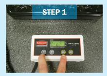
Turn scale on by pressing the lbs/kg button and ON buttons simultaneously
