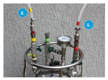
**1. Gas In:** The pressurization port (**RED**) remains in the open position for the duration of the injection.
