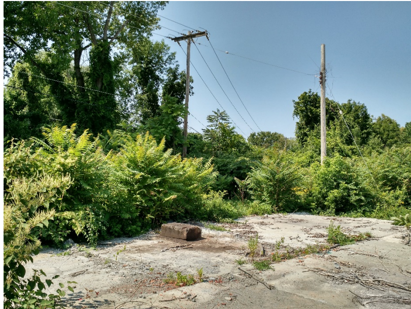
Surficial staining present at Surface Pedestal sample location where PCBs were detected
