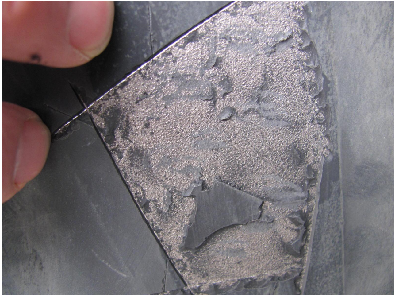
Photo 2 – Typical peened surface profile.
