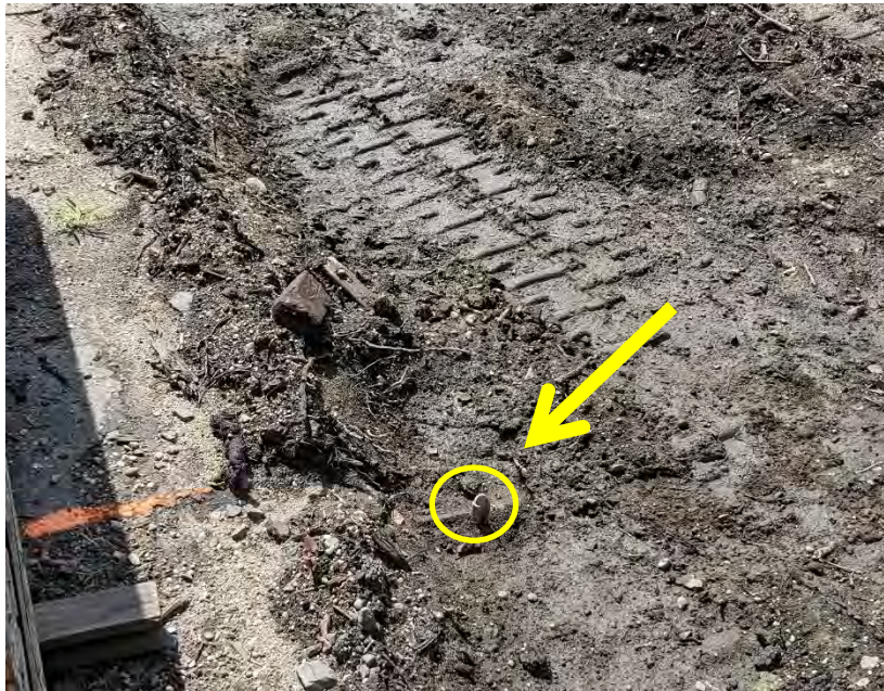
Photograph 13: View of the casing of MW1 during a previous visit on August 31, 2021, which was observed to be broken at the top.
