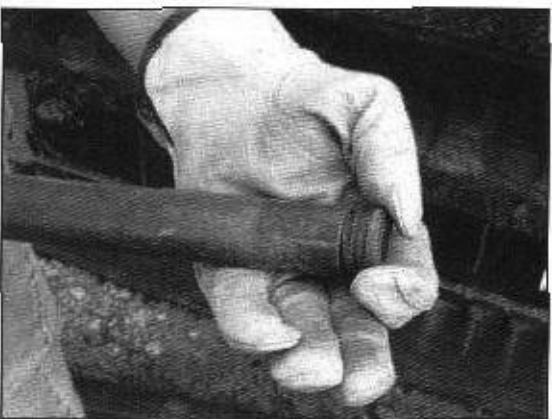
Figure 4.22. The MCS Plug is threaded onto the end of the 1.25-inch light-weight center rod.
