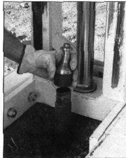
Figure 4.26. The pull cap is one way to remove the sampler from the ground.
