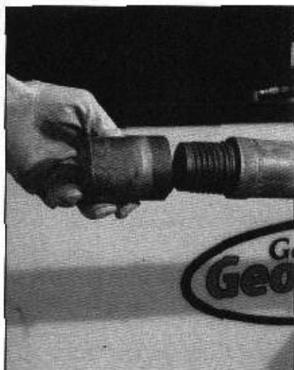
Figure 4.24. Place drive cap onto sampler drive head.
