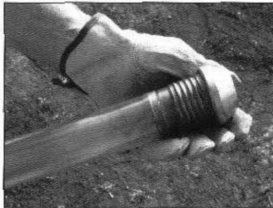
Figure 4.7. Place either end of the liner onto the extended shank cutting shoe. (This is used in place of a spacer ring or core catcher)
