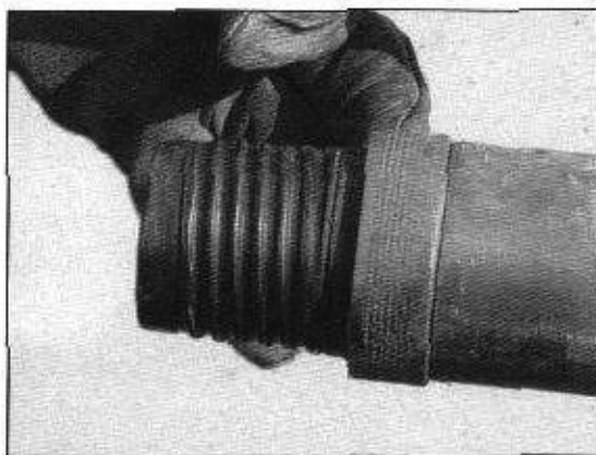
Figure 4.10. Thread the MC5 Drive Head onto the opposite end of the sample tube. Tighten by hand.
