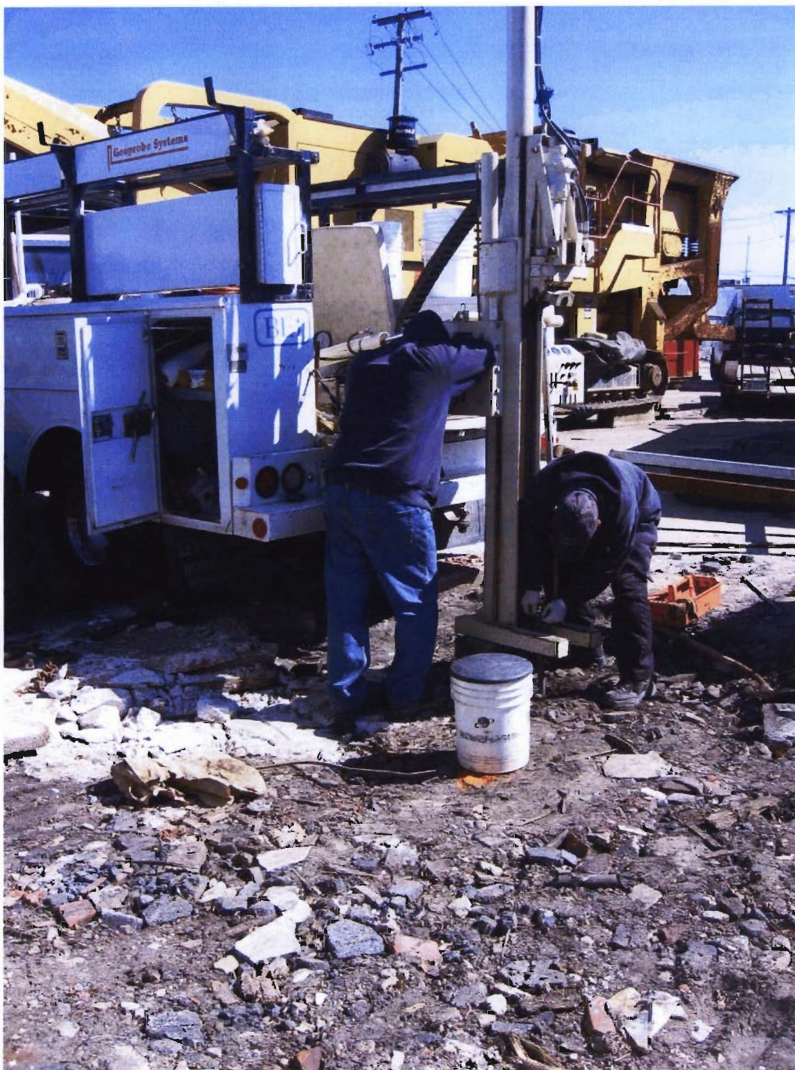
Photograph No. 7 - Supplemental soil sampling in subgrade soil source areas to collect samples for pre-disposal characterization for the IRM.
