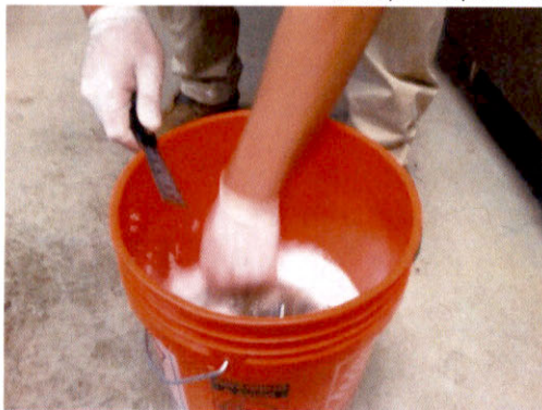
Adding sediment in the cup to surfactant solution.
