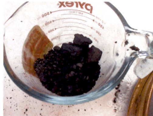
Transferring the >0.180 -mm washed sediment to a glass cup. The >2 -mm sediment on the left will also be transferred to the cup. The cup in the picture on the right contains both sizes of soil.
