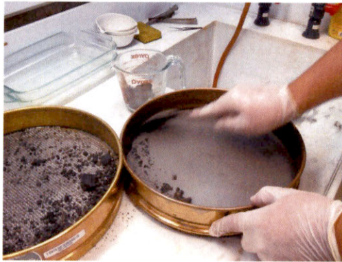
Transferring the >0.180 -mm washed sediment to a glass cup. The >2 -mm sediment on the left will also be transferred to the cup. The cup in the picture on the right contains both sizes of soil.
