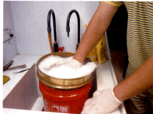
Hand scrubbing the <2 -mm fraction
