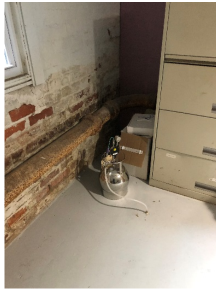
Photo #2: Sub-slab vapor sampling at 220 Lakeville Road (typical)
