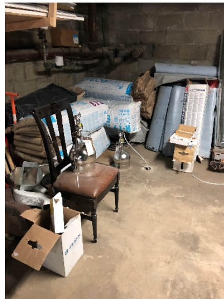
Photo #4: Concurrent indoor air and sub-slab vapor sampling at 218 Lakeville Road (typical)
