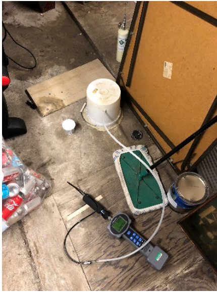
Photo #1: Representative view of helium test on sub-slab vapor probe
