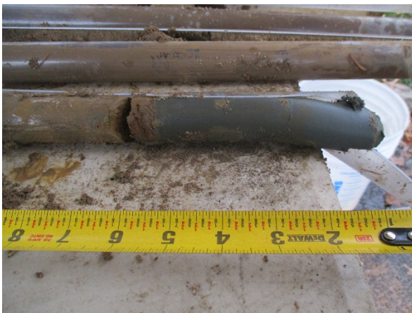
Photo #7 (11/12/2020): Contact between sand and clay at off-site monitoring well location PW-4
