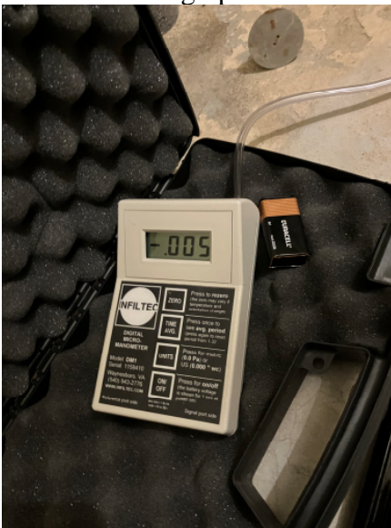
MP-02 reading under final operating settings (-0.005 in WC)
