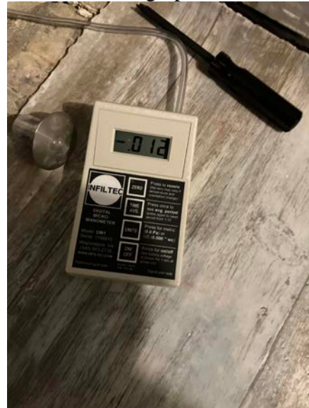
MP-03 reading under final operating settings (-0.012 in WC)
