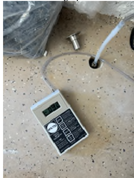
MP-01 reading under final operating setting (-0.092 in WC)
