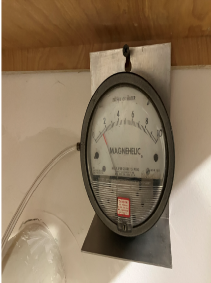
SSD-1 Pressure gauge (Dwyer Magnehelic)
