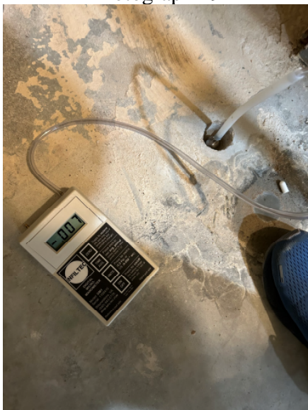
MP-02 reading under final operating settings (-0.007 in WC)
