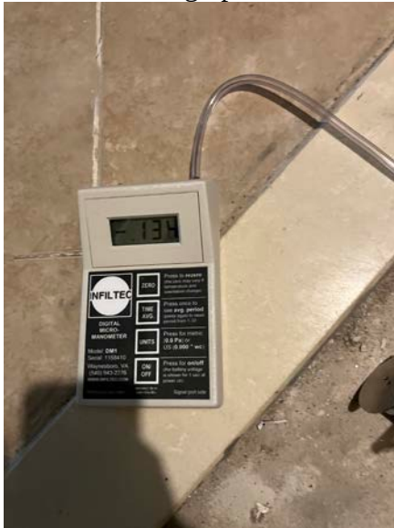
MP-01 reading under final operating settings (-0.134 in WC)
