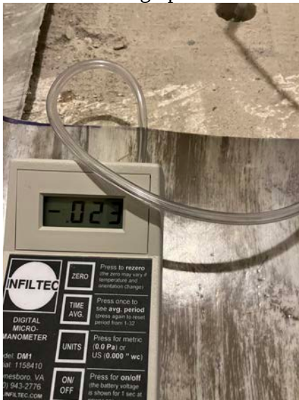
MP-04 reading under final operating settings (-0.023 in WC)
