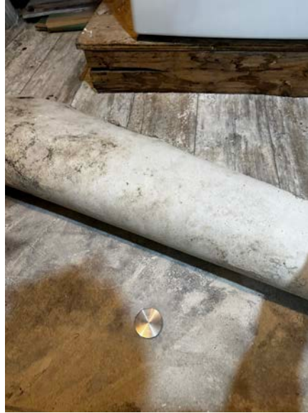
MP-01 stainless-steel vapor pin.
