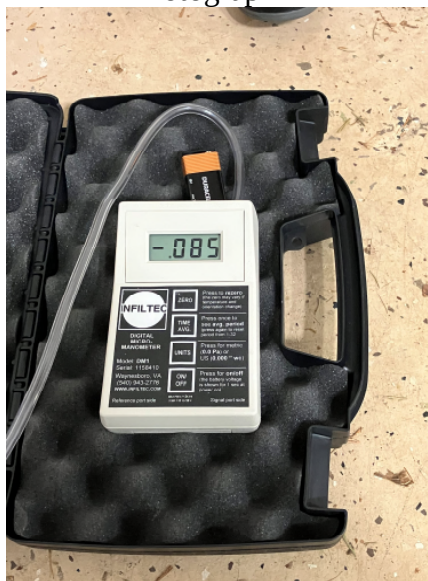
MP-01 reading under final operating settings (-0.085 in WC)
