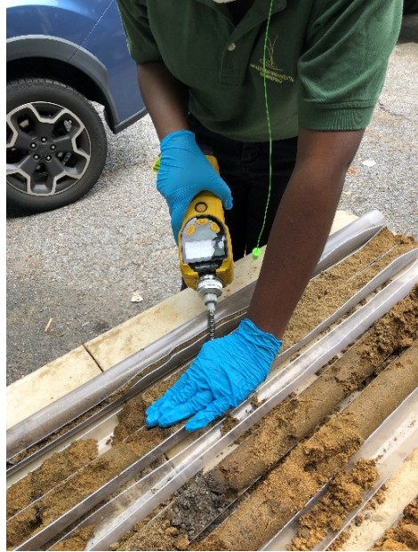
Photo #2 (8/31/2020): Field screening of soil borings with PID (typical)
