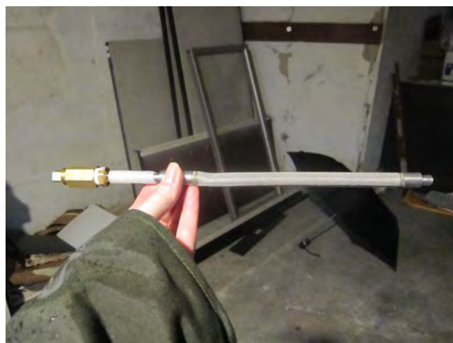
4. View of sub slab vapor sampling probe to be installed in a hole drilled through a building slab.
