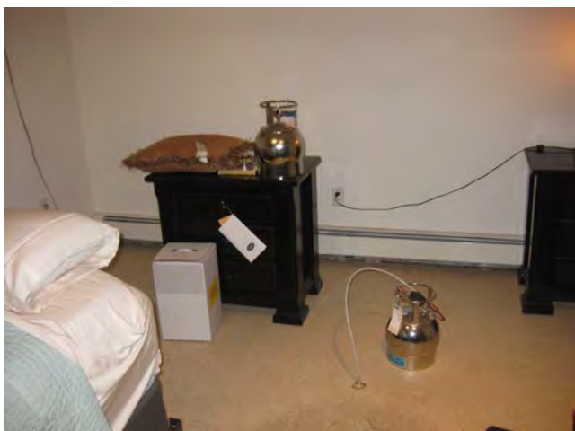
5. View of Summa canisters collecting indoor air and sub slab vapor samples (to be performed over a 24-hour time frame).
