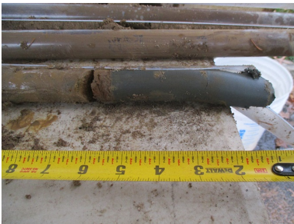
Photo #7 (11/12/2020): Contact between sand and clay at off-site monitoring well location PW-4
