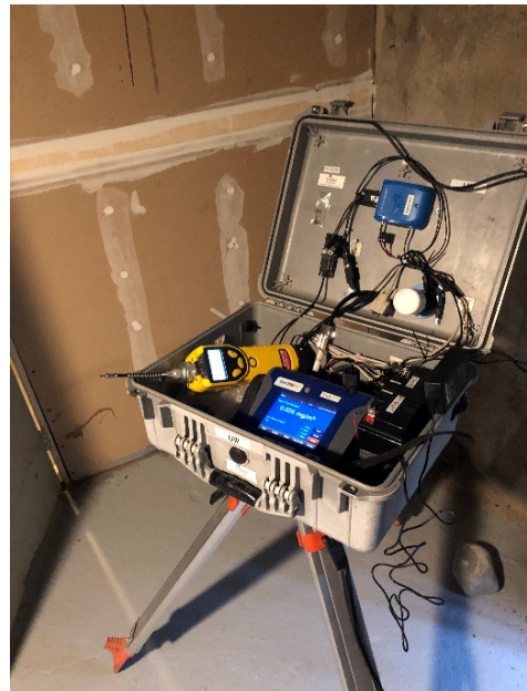
Photo #4 (9/1/2020): CAMP air monitoring equipment set up inside building
