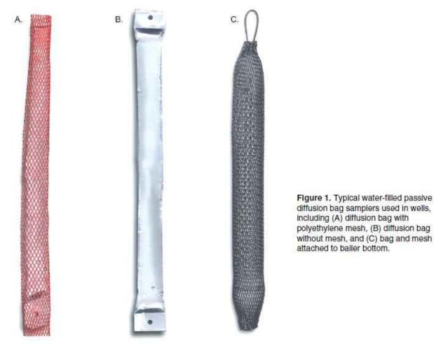
The PDB sampling method has several technical and logistical benefits compared to standard wellpurging methods; however, PDBs are not applicable for all contaminants or sites. See **Attachment 1** for ITRC's *Screening Worksheet for PDB Implementation*.
