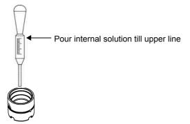
• Check air bubbles in a membrane cap.
