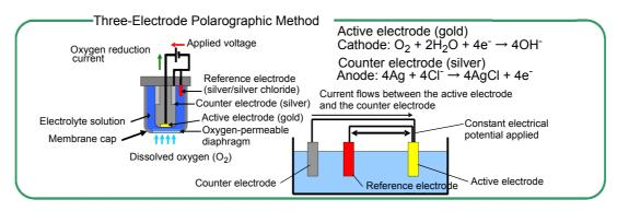
Fig. 1 Overview of principles behind dissolved oxygen sensor
