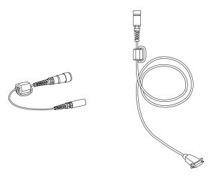
**Figure 19.2 Cables with Ferrite Beads**
