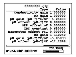
Figure 21.2 Calibration Record Screen 2
