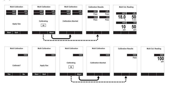
For a multi-sensor span calibration, a constant-flow regulator producing 0.5 to 1 liters per minute should be used, and the calibration cap must be installed on the instrument. Testing and calibration with an AutoRAE 2 must be performed using demand-flow regulators. A calibration cap must not be used. Teflon tubing must be used to test or calibrate the PID sensor. Follow the steps described here to perform a multi-sensor span calibration:
