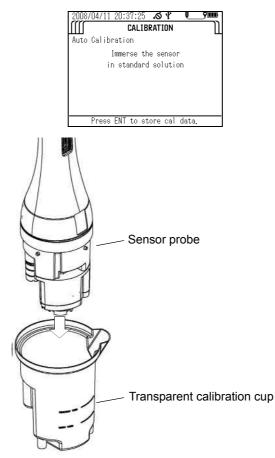
7. With the sensor probe still in the transparent calibration cup, place the transparent calibration cup into the black calibration cup.
