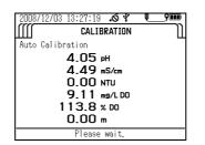
Calibration is finished when the message "Cal complete. MEAS to measure." appears. Press the MEAS key to set the measurement screen, then start measurement.
