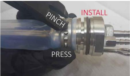
Figure 4-4: Installing the Bladder Clamp
