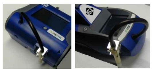
Figure 2-8: Installing Door-Oliver Cyclone
