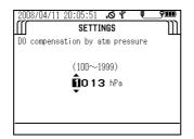
6. To save the change, press the up (△) and down (▽) keys to move the cursor to SAVE, then press the ENTER key. If you don't want to save the change, press the ESC key.
