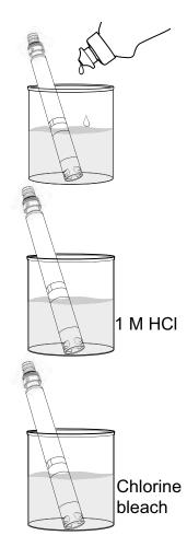
Figure 70 pH and pH/ORP sensor maintenance
