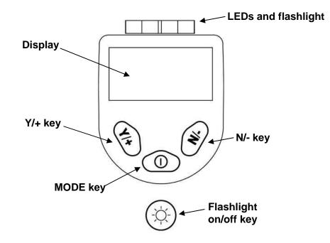
In addition to their labeled functions, the keys labeled Y/+, MODE, and N/- act as "soft keys" that control different parameters and make different selections within the instrument's menus. From menu to menu, each key controls a different parameter or makes a different selection.
