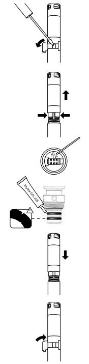
Figure 77 pH - pH/ORP sensor module replacement
