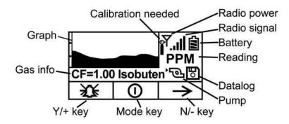
During sampling, the display's readings are shown numerically, plus the graph tracks the highest readings over time. The numeric reading alternates between the value and the measurement units, as well:
