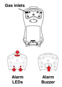
**Note:** The front of the diffusion model of the MultiRAE Lite is the same as the pumped model, but instead of a single gas inlet at the top, there are five inlets on the back side, as well as an extra alarm buzzer and LEDs.
