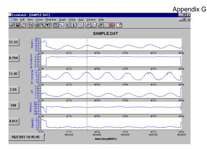
Note that the exact measurements for this point in time are displayed to the left of the graph. While holding down the right mouse button, move to another area on the graph. Notice how the measurements change as you move. When you release the mouse button, the display returns to normal.
