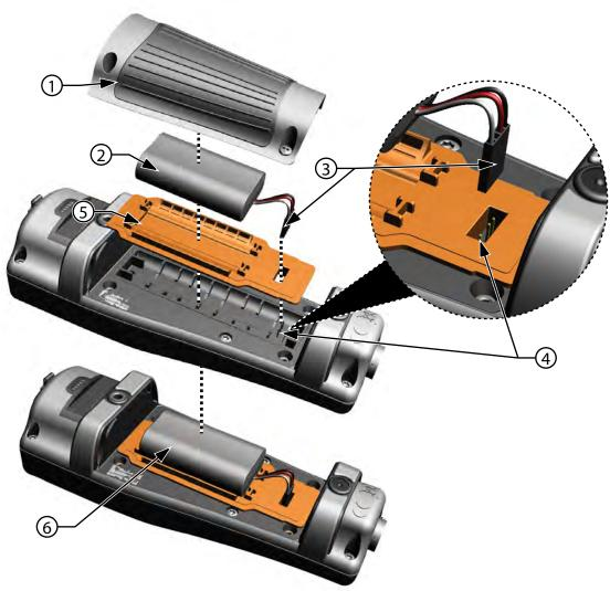
Figure 2 Battery replacement
