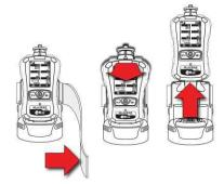
To secure: Press the MultiRAE into the cradle and fasten the Velcro strip.
