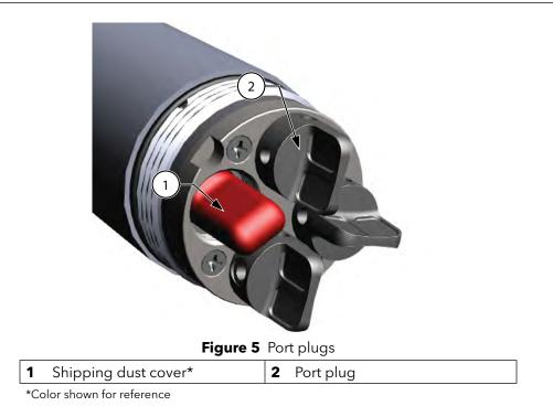
To protect the bulkhead connectors from damage, install a port plug into any port without an installed sensor. Port plugs and a tube of o-ring lubricant are included in the maintenance kit that ships with all ProDSS cables. Refer to the accessories section if an additional maintenance kit is needed (Ordering on page 73).
