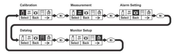
**Note:** When you reach Monitor Setup and press [N/-], the menu cycles back to Calibration.
