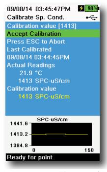
Figure 45 Calibrate specific conductance
