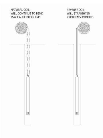
Figure 2-1: Reverse Coil Method
