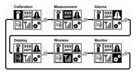
To enter a menu and view or edit parameters in its submenus, press [Y/+].
