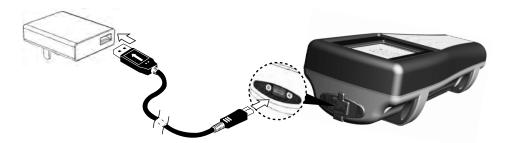
Figure 1 Connecting the ProDSS to AC power supply
