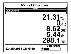
Figure 6.11 DO mg/L Calibration Screen
