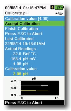
Figure 51 Calibrate pH 2- or 3-point
