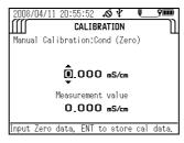
12. When the message "Cal complete. Press ENT to Span cal." appears, press the ENTER key to start the first span calibration procedure.
