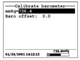
Figure 10.6 Barometer Calibration Screen
