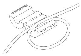
**Figure 19.1 Ferrite Bead Installation**
