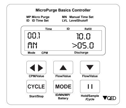
In User Set mode the CPM and UP, DOWN keys function differently than MP mode. The CPM key becomes a key used to select the digits of the refill and discharge time settings found at the rightmost positions on the display. The UP and DOWN keys are used to adjust the digit value up or down. By selecting and adjusting digits up and down a user can quickly set any time from 00.1 seconds to 99.9 seconds. Sampling in User Set mode is the same as explained, above, for MP mode.
