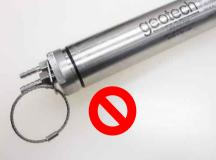
Figure 4-16a: Incorrect Installation
