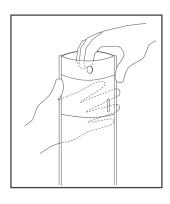
**1** Remove HydraSleeve from package and grasp top to "pop" open. Remember to save the discharge tube for later.
