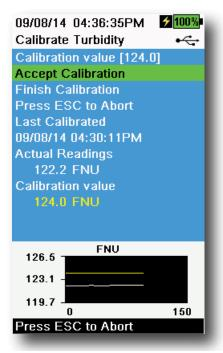
Figure 54 Calibrate turbidity
