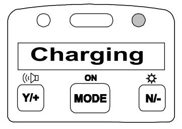
5. When the battery is fully charged, the LED will change from red to green and the message "Fully charged" will appear on the display. After the battery is fully charged, the unit will enter the "trickle charge" mode. In which, the red LED will turn on for several seconds every minute, to maintain the full charge.
