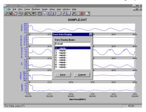
Then type "Default" for the file name and click **Save**. The parameters, colors, format, and x-axis time interval associated with the current display are now saved and can be accessed any time in the future. Nine different data displays may be saved for any data file. You can easily switch between various displays of the data. The data files can be accessed by clicking **Load Data Display** from the file menu and then selecting the desired presentation.
