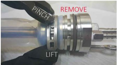
Figure 4-2: Removing the Bladder Clamp
