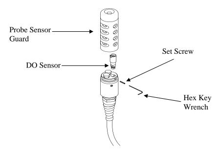
Figure 11.1 DO Sensor Replacement
