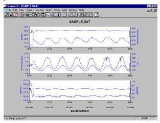
Click **1 Trace per Graph** to return the display to the original setting. Move the cursor to any position in the graph, then click and hold the right mouse button.
