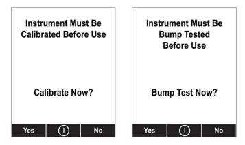
If "Can't Bypass" is selected, the display looks like this, and only allows the options of performing the test or shutting down:
