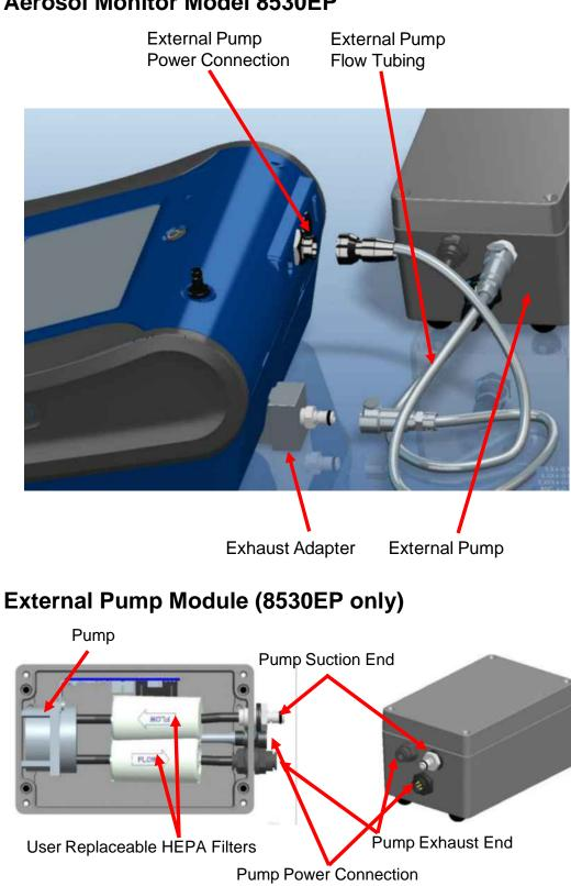
Parts Identification for the DustTrak II Desktop Aerosol Monitor Model 8530EP
