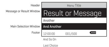
As described previously, the **EXIT** button allows an exit or escape from the current menu and a return to the previous menu. This allows a rapid exit from an inner menu to the main menu by repeatedly pushing the **EXIT** button. Pushing **W** at any time will turn the 2020t/i off.
