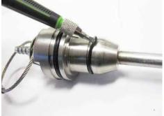
Figure 4-5: Removal of O-rings
