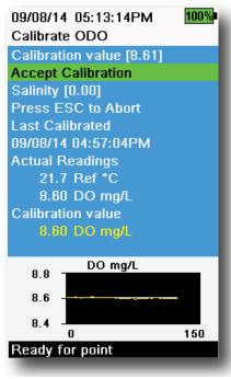
Figure 48 Calibrate ODO mg/L
