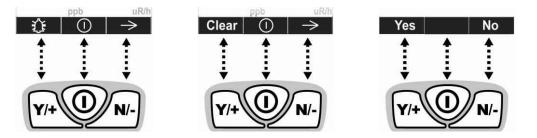
In addition to the functions described above, any of the keys can be used to manually activate display backlighting. Press any key when the backlighting is off to turn it on. A subsequent key press is required to carry out an actual function corresponding to that key.
