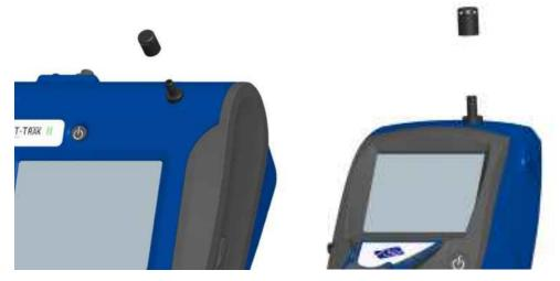
The inlet cap can simply be pressed onto the instruments inlet.
