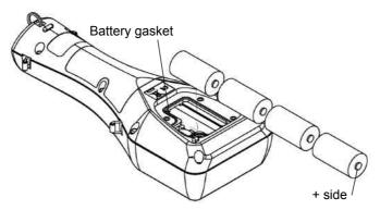
*4.* Replace the battery cover and fasten it with the 4 screws. Tighten the screws to less than 0.5 N·m.
