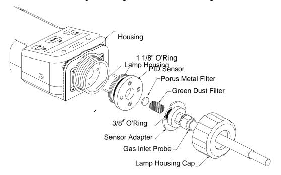
Figure 7-2 Sensor Components
