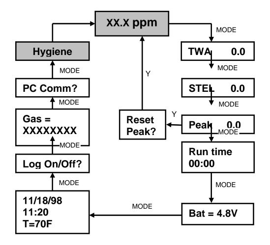
To choose a specific display, press the [MODE] key one or more times until the desired display appears, or the [Y/+] key where indicated with a Y.
