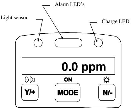
Figure 2-2 LCD Display and Keypad
