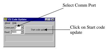
**9.** Set the Comm port number to match the port that you connected the 655173 PC Interface Cable to, then click on the Start Code Update button.
