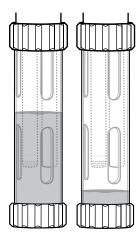
Figure 63 Conductivity/Temperature Short-term storage
