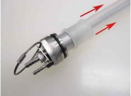
Figure 4-3: Removal of upper Compression Ring
