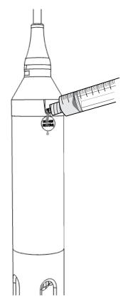
Figure 59 Depth sensor flush
