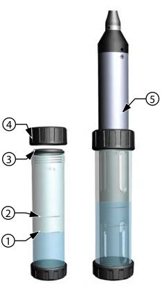
Figure 44 Calibration cup standard volume
