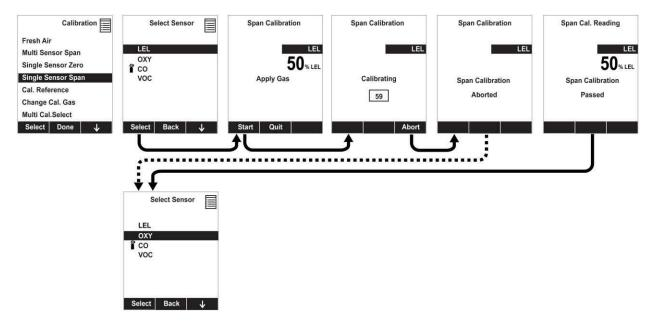
After a timer countdown, the span calibration is done. The LCD will display whether the calibration was successful and the reading for that calibration gas.
