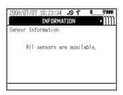
• When there is a sensor probe problem, individual measurement parameters generate messages such as the one shown below. Follow the troubleshooting information to remove the problem before continuing to operate the system.
