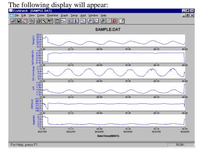
Note that the data in this file appears as a graph of temperature, specific conductance, dissolved oxygen, pH, ORP, and depth, all versus time. The graphs are scaled automatically so that all data fits comfortably on the computer screen. Note also that this data file was obtained with a 6-series sonde for which a depth sensor is available. Depth is NOT a current parameter for the 556 MPS.
