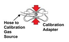
Grasp the small handles on the Calibration Adapter.
