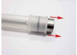
Figure 4-2: Removal of bottom Compression Ring
