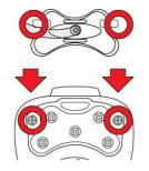
Align the Calibration Adapter's two connectors with the screws on both sides of the MultiRAE's gas inlets.
