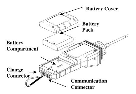
Figure 6-1 Battery Replacement
