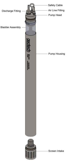
Figure 1-2: Basic\* Bladder Pump Assembly
