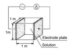
Fig. 3 Definition of conductivity
