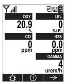
Five sensors, including Gamma radiation sensor.
