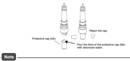
Before measuerment, remove the rubber cap (whit) and the protective cap (blk).
