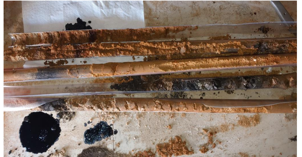
32. View of soil cores from SB-5 (minus oil splotch from previous location)
