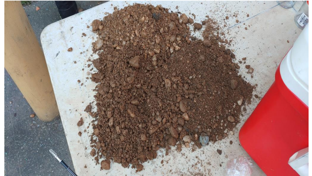
18. Soil from hand auger SB-2 at 0.5-5 feet
