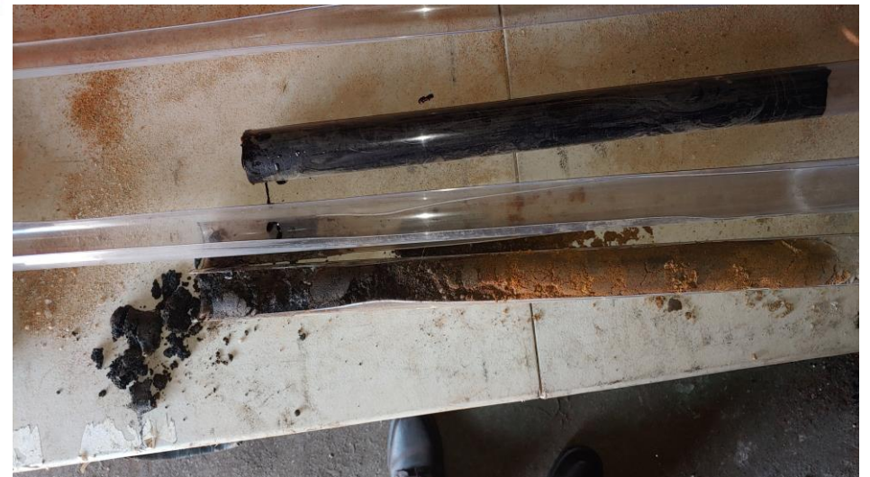
28. Soil core and sample full of oil at SB-4
