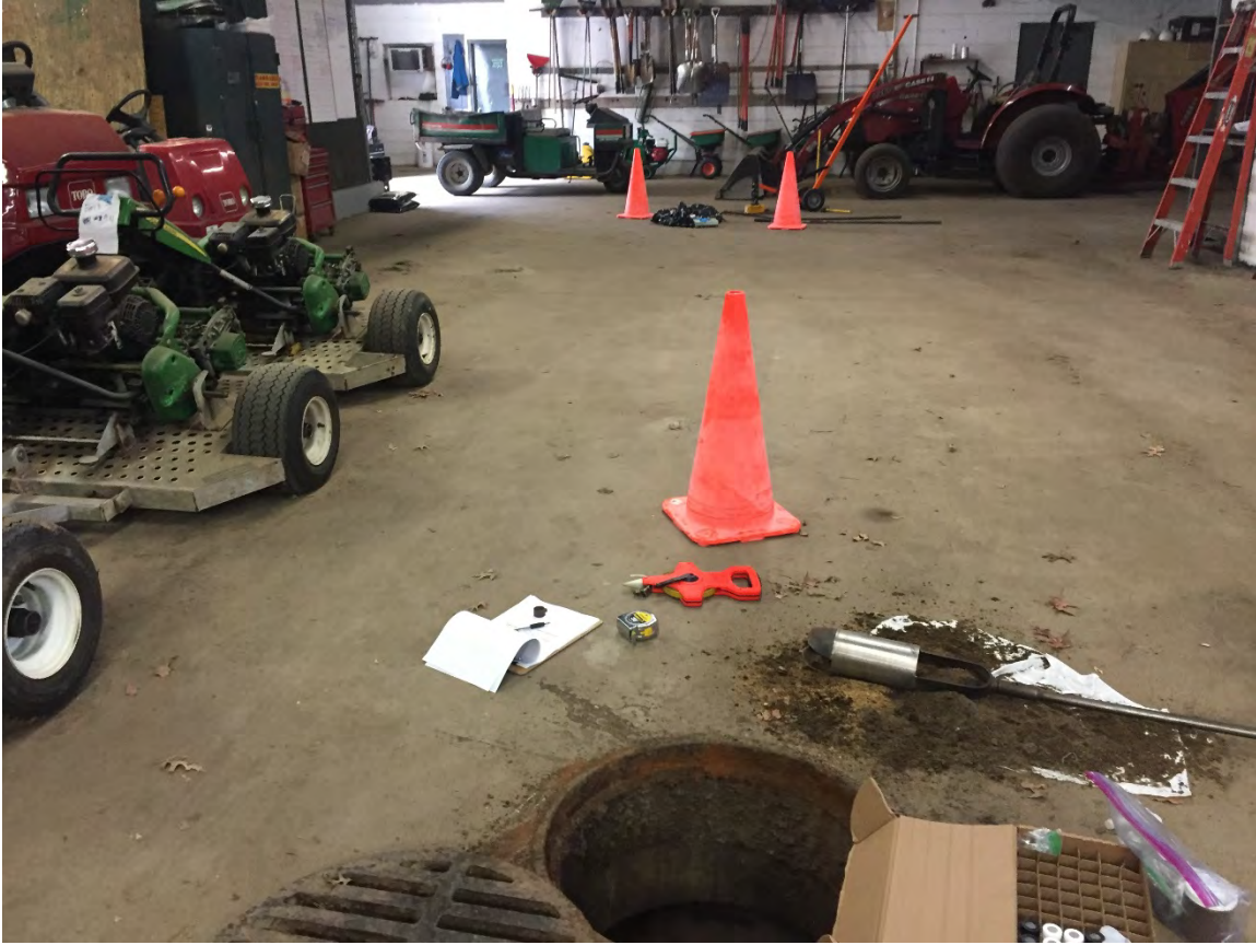
Photograph No. 11: The collection of a sediment sample from an interior floor drain.
