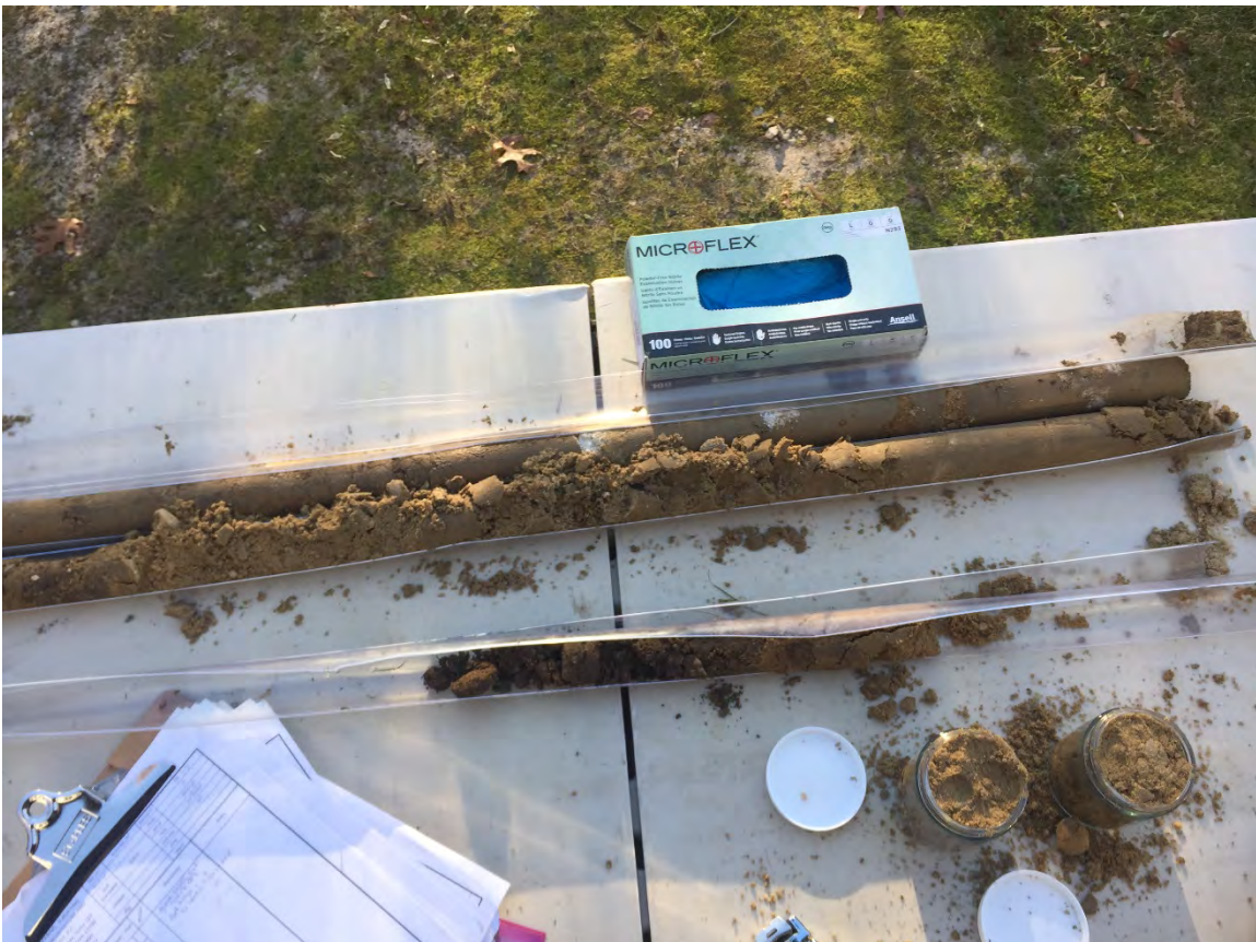
Photograph No. 10: Typical soil boring core and soil sample collection from the same.
