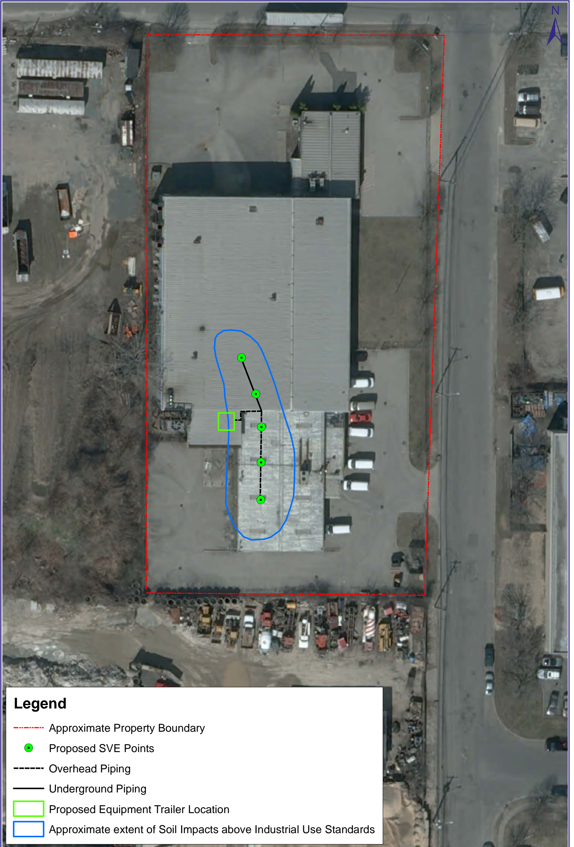
FIGURE 5-1 ALTERNATIVE 1 - RESTORATION TO INDUSTRIAL USE SOIL VAPOR EXTRACTION FORMER BARON BLAKESLEE SITE BAY SHORE, NEW YORK
