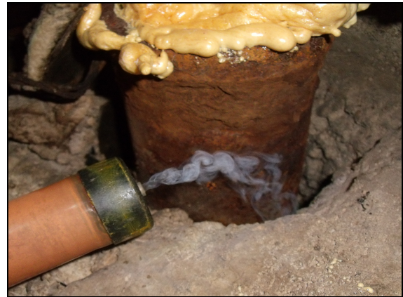
Photo #4: Air flow into restaurant from dry cleaner basement.
