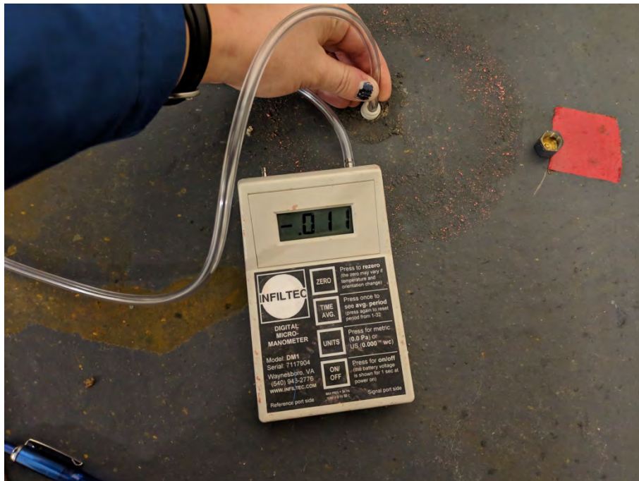
8. Negative pressure reading at VEMP-2 (northeastern portion of building)
