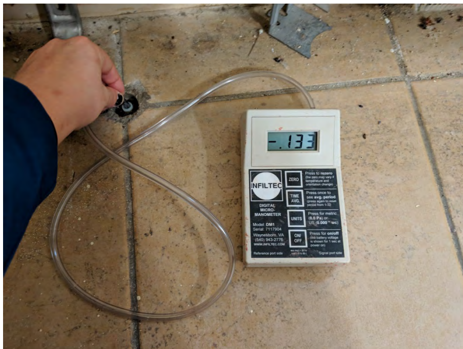
10. Negative pressure reading at VEMP-4 (southeastern portion of building)
