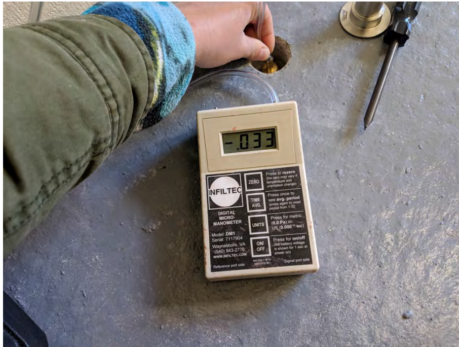
7. Negative pressure reading at VEMP-1R (northwestern portion of building)
