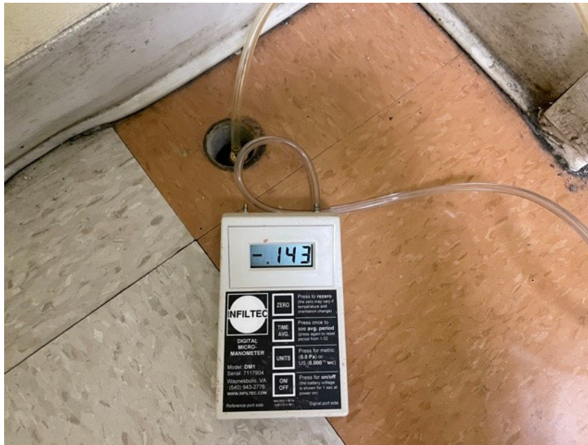
11. Negative pressure reading at VEMP-3R (southwestern portion of building)
