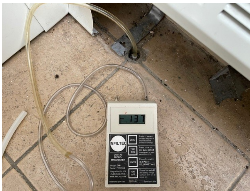
12. Negative pressure reading at VEMP-4 (southeastern portion of building)
