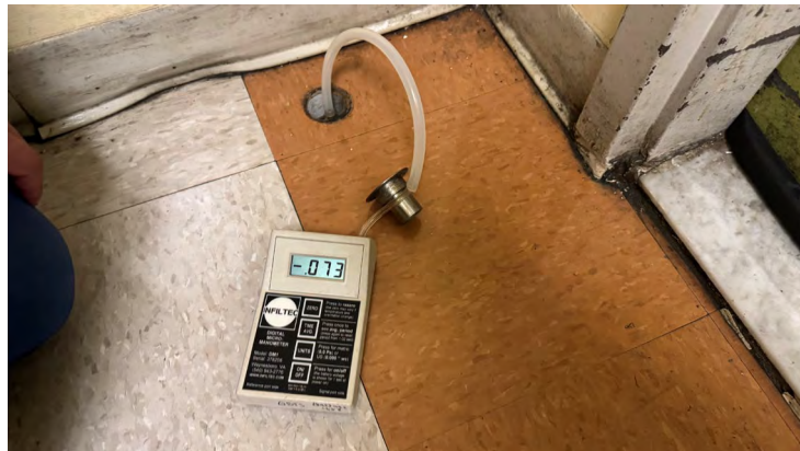
11. Negative pressure reading at VEMP-3R, southwestern portion of building
