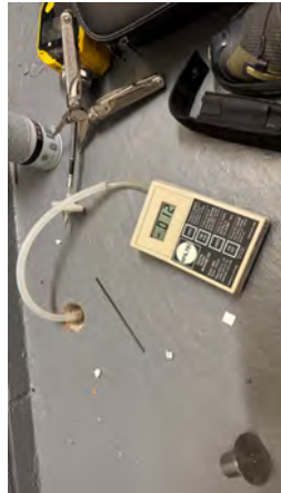
9. Negative pressure reading at VEMP-1R, northwestern portion of building
