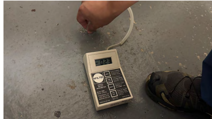
10. Negative pressure reading at VEMP-2, northeastern portion of building
