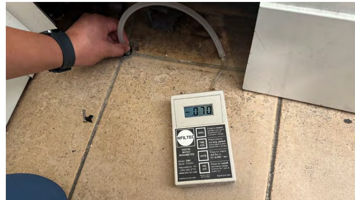
12. Negative pressure reading at VEMP-4, southeastern portion of building
