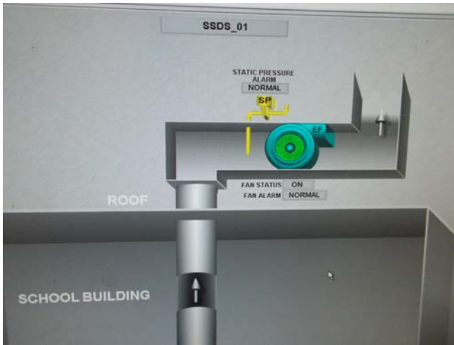
Photo 1: View of BMS on typical SSDS fan unit (EF-1).
