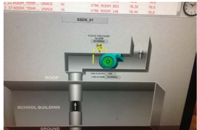
Photo 2: View of typical BMS showing normal status on SSDS fan unit SSDS-1.
