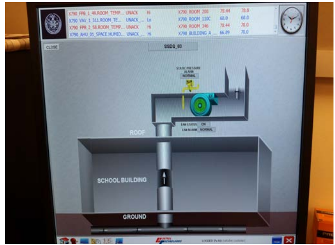
Photo 2: View of functional BMS associated with SSDS fan unit EF-3.
